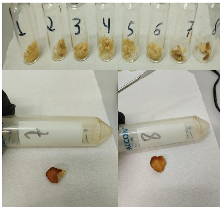
Figure S16. Kinetics of delignification, showing the solid fraction obtained at different reaction times: (1) 30 min, (2) 45 min, (3) 60 min, (4) 90 min, (5) 120 min, (6) 180 min, (7) 270 min, and (8) 360 min. Conditions: DGDE molar fraction = 0.1 (ET predominance), T = 100 \pm 1 °C, [PTSA] = 0.03 M, S/L = 1:10.
