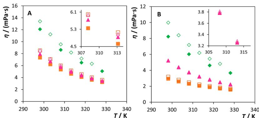
**Figure 7.** Experimental viscosity as a function of temperature for ternary mixtures identified in Table 2 as TL1 (full symbols) and TL2 (open symbols):  $[\text{C}_4\text{mim}][\text{SCN}] + \text{KCH}_3\text{CO}_2$  (orange ■);  $[\text{C}_4\text{mim}][\text{SCN}] + \text{NaCH}_3\text{CO}_2$  (red ▲);  $[\text{C}_4\text{mim}][\text{N}(\text{CN})_2] + \text{KCH}_3\text{CO}_2$  (green ◆). A, IL-rich phase; B, salt-rich phase.
