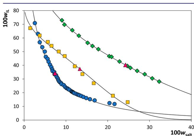
**Figure 2.** Ternary phase diagrams for ABS composed of IL +  $\text{KCH}_3\text{CO}_2 + \text{H}_2\text{O}$ :  $[\text{C}_4\text{mim}][\text{CF}_3\text{SO}_3]$  (blue ●);  $[\text{C}_4\text{mim}][\text{SCN}]$  (yellow ■);  $[\text{C}_4\text{mim}][\text{N}(\text{CN})_2]$  (green ◆); critical point (red ▲); adjusted binodal using eq 1 (—).
