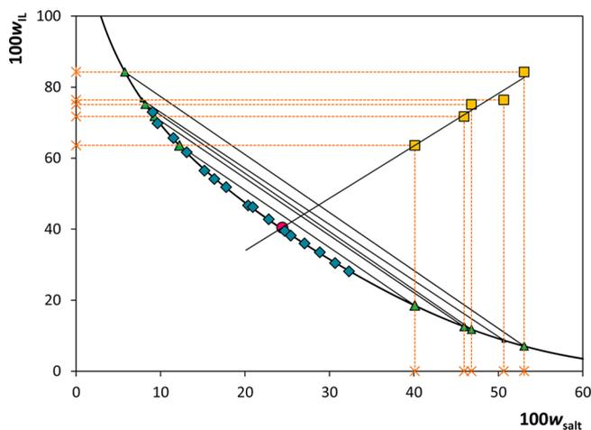
**Figure 5.** Phase diagram for the ternary system composed of [C<sub>4</sub>mim][N(CN)<sub>2</sub>] + KCH<sub>3</sub>CO<sub>2</sub> + H<sub>2</sub>O: binodal curve data (blue  $\blacklozenge$ ); adjusted binodal data through eq 1 (—); TL data (green  $\blacktriangle$ ); TLs relation (yellow  $\blacksquare$ ); critical point (red  $\bullet$ ).
