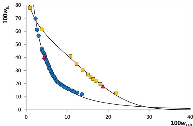
**Figure 3.** Ternary phase diagrams for ABS composed of IL +  $\text{NaCH}_3\text{CO}_2 + \text{H}_2\text{O}$ :  $[\text{C}_4\text{mim}][\text{CF}_3\text{SO}_3]$  (blue ●);  $[\text{C}_4\text{mim}][\text{SCN}]$  (yellow ■); critical point (red ▲); adjusted binodal using eq 1 (—).
