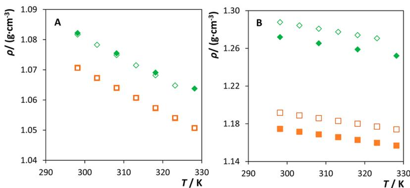
**Figure 9.** Experimental density as a function of temperature for ternary mixtures identified in Table 2 as TL1 (full symbols) and TL2 (open symbols):  $[\text{C}_4\text{mim}][\text{SCN}] + \text{KCH}_3\text{CO}_2$  (orange ■);  $[\text{C}_4\text{mim}][\text{N}(\text{CN})_2] + \text{KCH}_3\text{CO}_2$  (green ◆). A, IL-rich phase; B, salt-rich phase.
