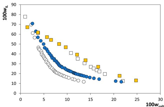
**Figure 4.** Evaluation of salt effect on the formation of [C<sub>4</sub>mim]-[CF<sub>3</sub>SO<sub>3</sub>]- (blue ●) and [C<sub>4</sub>mim][SCN]-based ABS (yellow ■): KCH<sub>3</sub>CO<sub>2</sub> (full symbols) and NaCH<sub>3</sub>CO<sub>2</sub> (open symbols).
