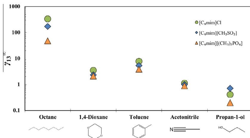
**FIGURE 3.** Infinite dilution activity coefficients of selected solutes in ILs, at  $T = 398.15$  K for propan-1-ol, and  $T = 358.15$  K for the other organic compounds.
