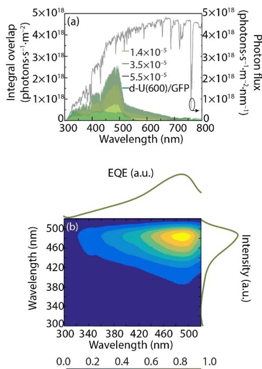
**Fig. 3** (a) Integral overlap between the solar photon flux and the absolute absorbance for each one GFP-based sample. The solar photon flux on Earth at AM1.5G is also presented (right y axis). (b) Cross correlation between the EQE of the PV cell coupled to the p-LSC based on the  $5.5 \times 10^{-5}$  M solution and its excitation spectrum. The colour-scale intensity is a measure of the correlation.
