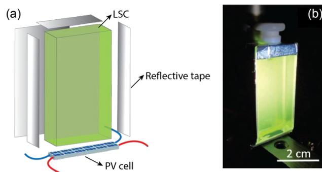
**Fig. 1** (a) Schematic representation of the p-LSCs and (b) photograph of the p-LSC based on a glass container filled with eGFP with concentration of  $5.5 \times 10^{-5}$  M, under AM1.5G illumination. The PV cell is located at the bottom edge.
