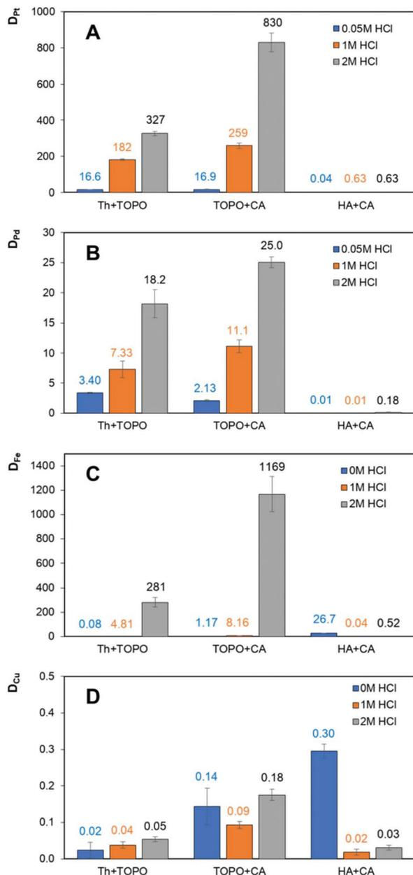
**Fig. 2** Distribution coefficient of Pt<sup>4+</sup>, Pd<sup>2+</sup>, Fe<sup>3+</sup> and Cu<sup>2+</sup> as a function of HES selection and HCl concentration ([Pt<sup>4+</sup>] = [Pd<sup>2+</sup>] = 2 mM; [Fe<sup>3+</sup>] = [Cu<sup>2+</sup>] = 10 mM; O : A = 0.5; 1 : 1 HES molar composition).
