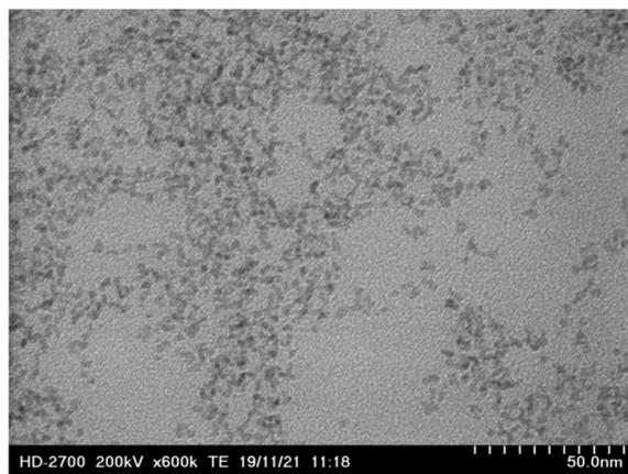
**Fig. 8** TEM analysis of the palladium nanoparticles obtained from the loaded Th + TOPO phase after coming into contact with a 0.1 M  $\text{NaCH}_3\text{COO}$  aqueous solution (contact time = 72 h, O : A = 0.5,  $x_{\text{TOPO}}$  = 0.5).
