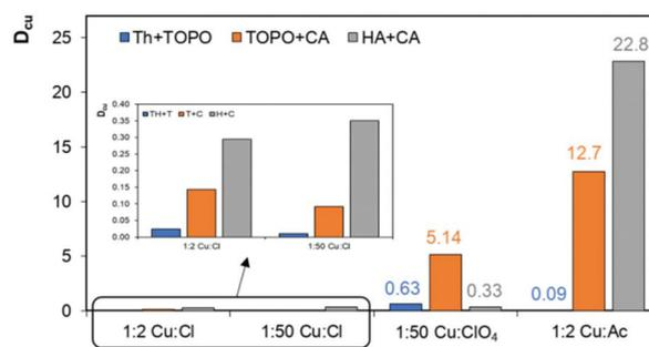
Fig. 3 Distribution coefficient of  $\text{Cu}^{2+}$  as a function of HES selection and sodium salt addition ( $[\text{Cu}^{2+}] = 10 \text{ mM}$ ; O : A = 0.5; 1 : 1 HES molar composition, pH = 4.9).
