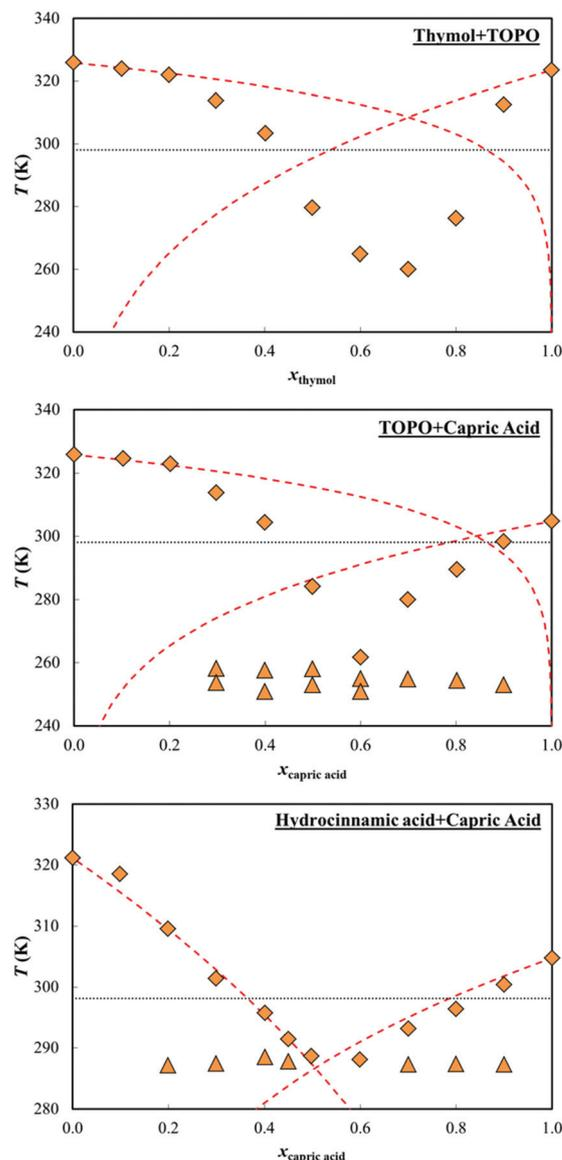
**Fig. 1** Phase diagram for the studied mixtures:  $\blacklozenge$  melting temperatures,  $\blacktriangle$  eutectic temperatures,  $---$  ideal solubility lines, and  $\cdots$   $T = 298.15$  K.
