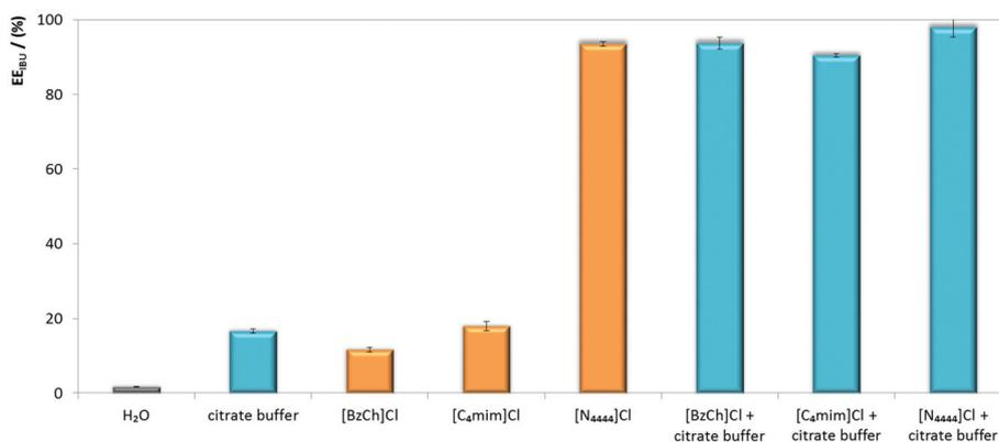
**Fig. 3** Extraction efficiencies of ibuprofen ( $EE_{IBU}$ , %) achieved in the solid–liquid extractions carried out with aqueous solutions of three ionic liquids (45 wt%) in the absence (orange bars) and presence (blue bars) of 5 wt% of citrate buffer. The data obtained for the experiments with water and citrate buffer at 5 wt% are depicted for comparison purposes.
