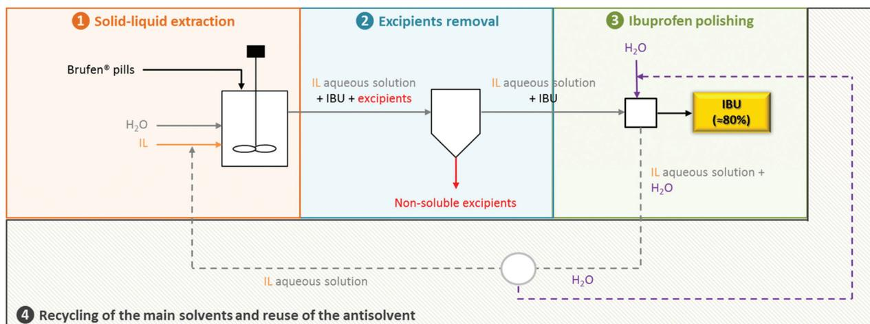
Fig. 2 Schematic representation of the integrated process of extraction, purification, ibuprofen recovery and recycling of the main solvents based on the use of aqueous  $[\text{N}_{4444}]\text{Cl}$  solution and water as the solvent and anti-solvent, respectively.
