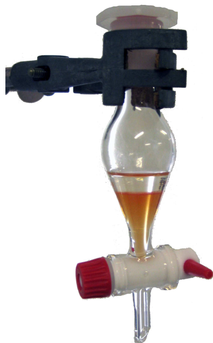
Fig. S5 Macroscopic evidence for the preferential partitioning of \beta -carotene for the bottom [\text{C}_4\text{mim}][\text{CF}_3\text{SO}_3] -rich phase (40 wt % of [\text{C}_4\text{mim}][\text{CF}_3\text{SO}_3] + 25 wt % of D-maltitol + 35 wt % of water).
