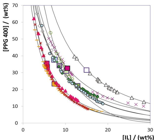
**Figure 2.** Phase diagrams for ABS composed of PPG 400 + IL + H<sub>2</sub>O at 25°C: [Ch][DHP] (—); [Ch][Ac] (▲); [Ch][Bit] (×); [Ch][DHCit] (△); [Ch]Cl (◆); [Ch][Prop] (◇); [Ch][But] (○); [Ch][Gly] (\*); [Ch][Lac] (●), with the corresponding fitting of the experimental data using Eq. (1) (—) and critical points (■).
