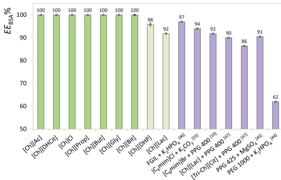
**Figure 3.** Average extraction efficiencies of BSA ( $EE_{BSA}$ %) in the systems composed of PPG 400 (30 wt%) + IL (30 wt%) + H<sub>2</sub>O (at least three replicates for each system were accomplished). Experiments were carried out in samples with a total of 3 g at 25°C and pH 7.4. BSA at an initial concentration of 0.5 g L<sup>-1</sup> was used. The comparison with literature results is also included.
