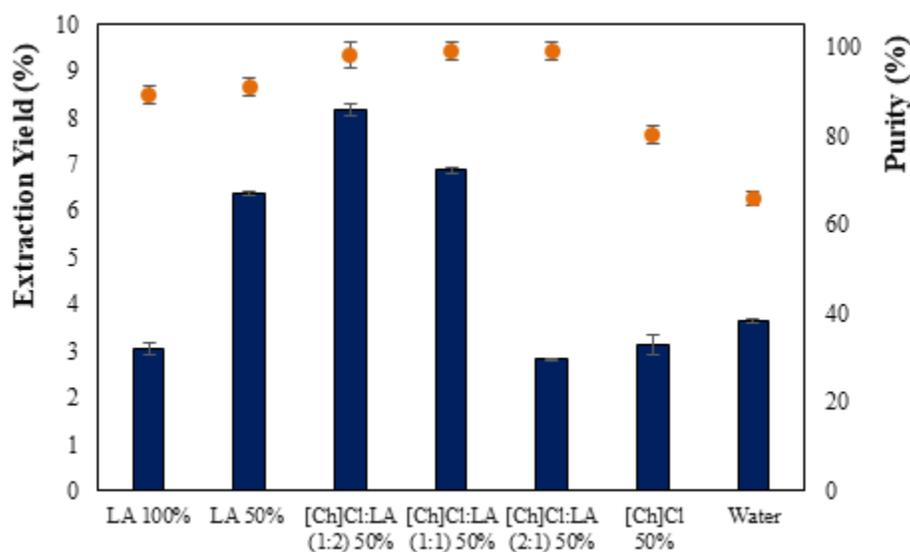
**Figure 4.** Extraction Yield (■) and Purity (●) of levodopa using lactic acid, aqueous solutions of lactic acid and aqueous solutions of ES based on LA (T = 50°C, S:L = 1:10, time = 90 min).
