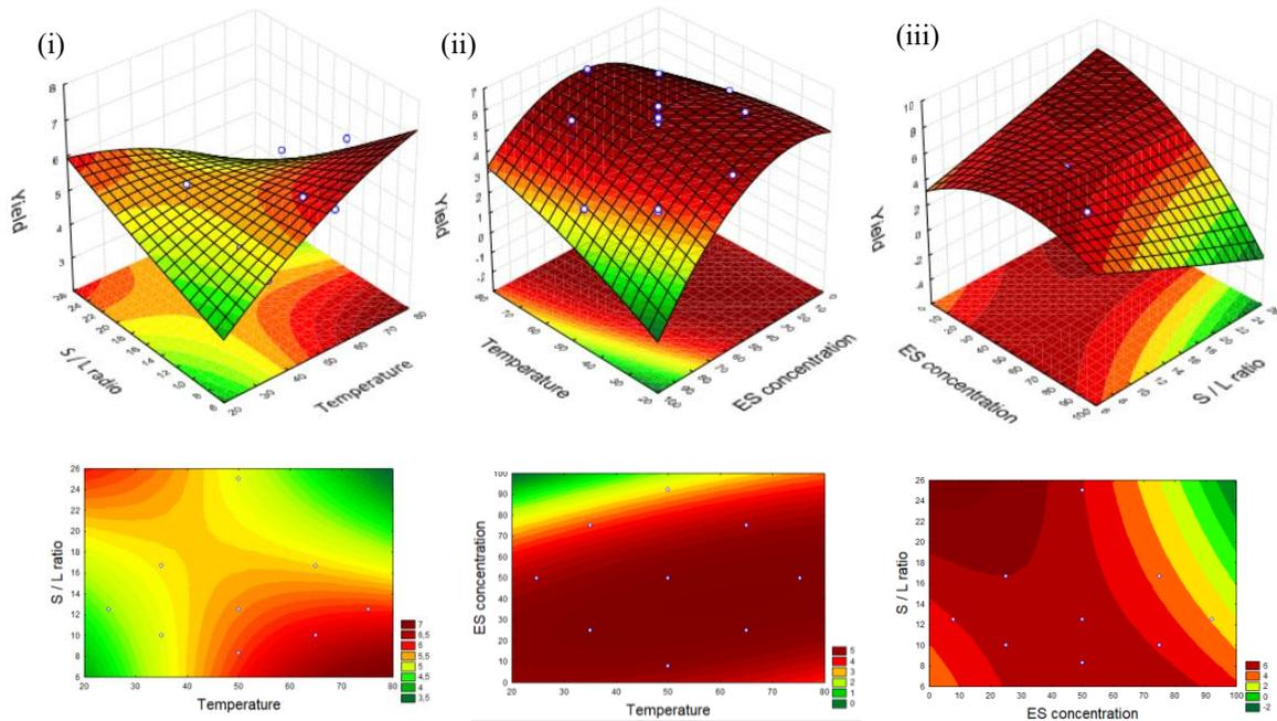
**Figure 5.** Response surface graphs on the levodopa extraction yield with the combined effects of (i) Temperature and S:L ratio, (ii) ES concentration and S:L ratio, (iii) Temperature and ES concentration using aqueous [Ch]Cl:LA (1:2) solutions for 90 minutes of extraction time.
