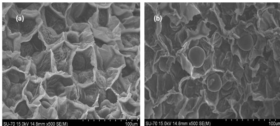
**Figure 8.** SEM images of the *Mucuna pruriens* samples after extraction with (a) water and (b) an aqueous solution of [Ch]Cl:LA (1:2).
