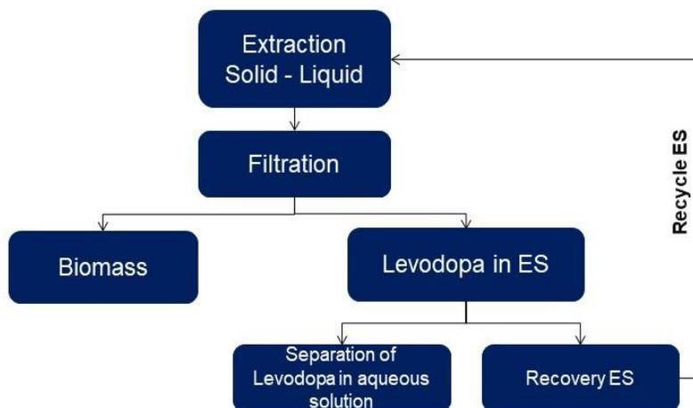
**Figure 7.** Flowchart for the extraction and separation of levodopa from *Mucuna pruriens* seeds.
