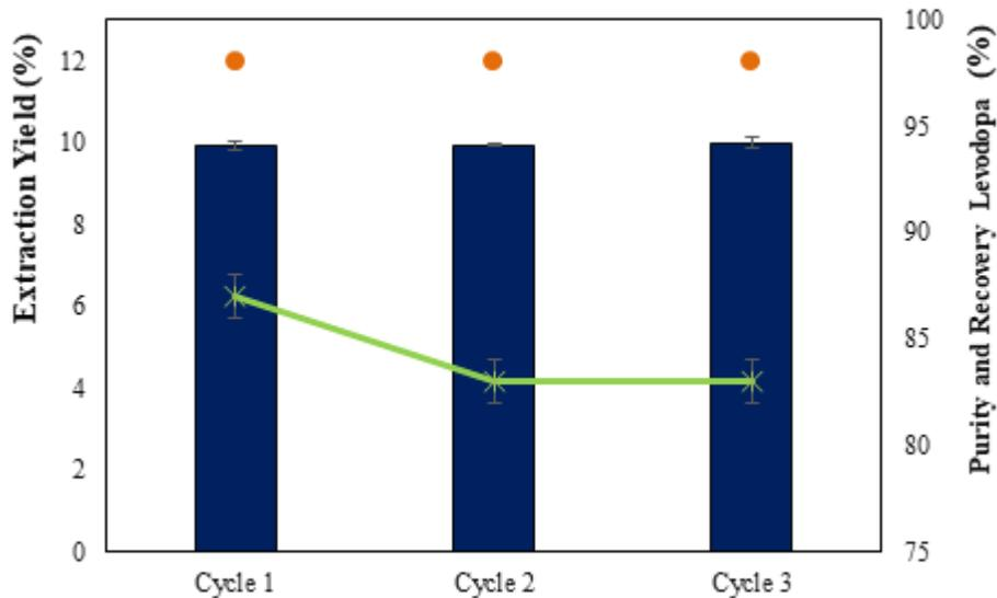
**Figure 6.** Results of Extraction Yield (■), Recovery (\*), and Purity (●) of Levodopa using the ES [Ch]Cl:LA (1:2) aqueous solutions at the optimized conditions and a cation exchange column for levodopa recovery.
