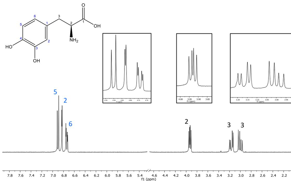
**Figure 9.**  $^1\text{H}$  NMR spectra of the recovered levodopa from  $[\text{Ch}]\text{Cl}:\text{LA}$  (1:2) aqueous solutions.
