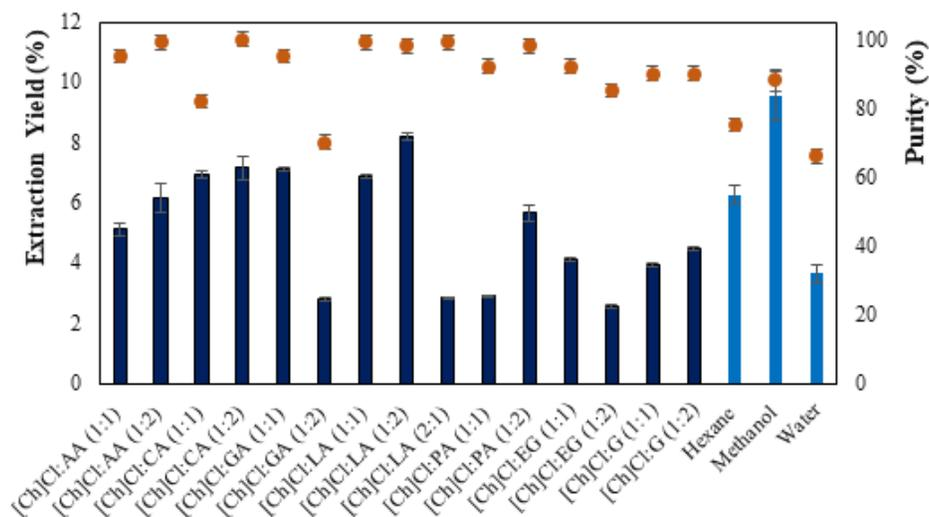
**Figure 3.** Extraction Yield (■) and Purity (●) of levodopa using aqueous solution of ES at 50 wt.% and Extraction Yield (■) and Purity (●) using hexane, methanol and water (T = 50°C, S:L = 1:10, time = 90 min).
