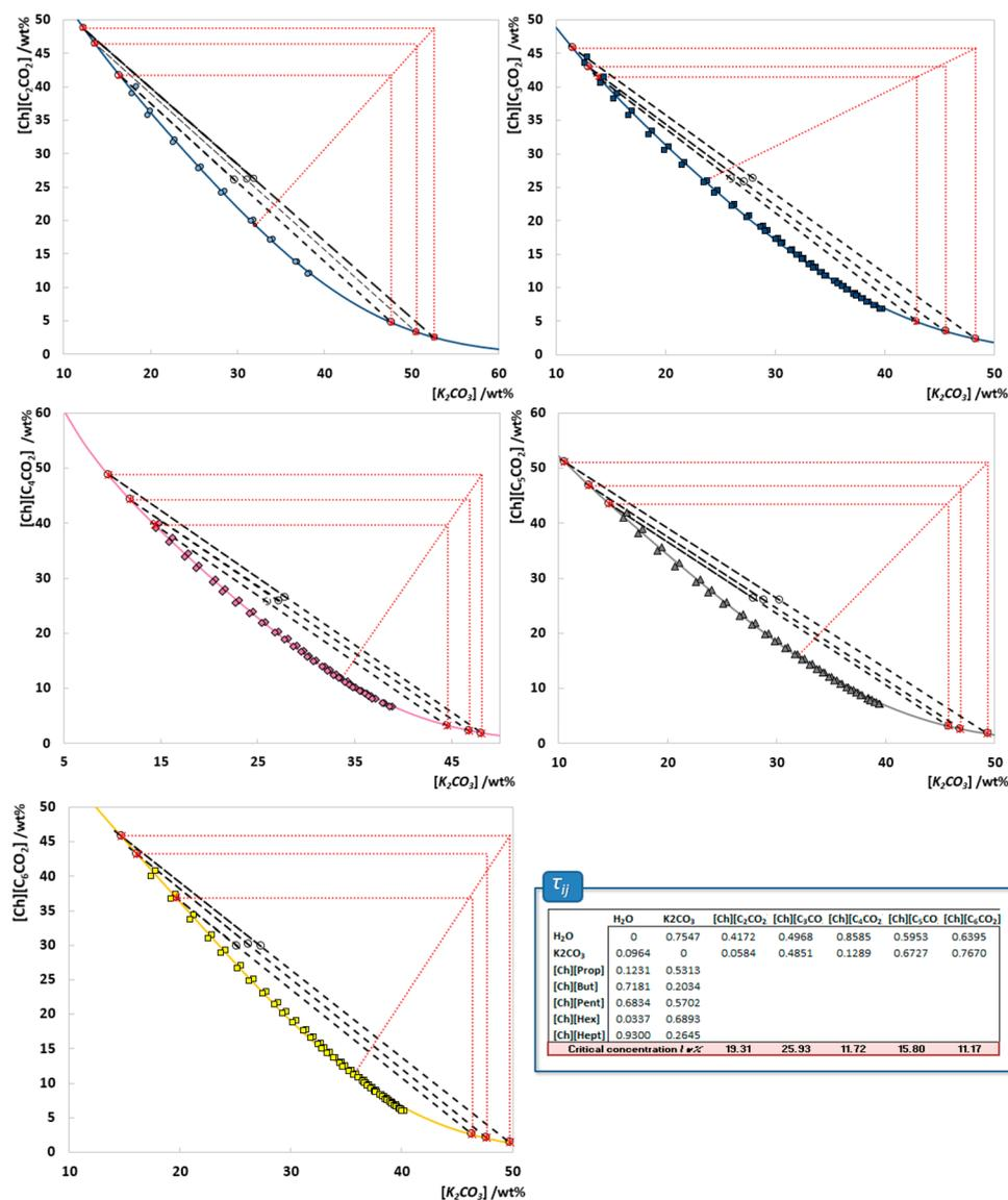
**Figure 3.** Phase diagrams for the studied ternary systems, optimized NRTL binary interaction parameters, and IL critical concentration: (Solid lines) fitting by eq 1; (red dotted lines) critical point estimation determined by eq 13; (black empty circles) experimental TLs; (red stars) TLs obtained from the NRTL fitting.
