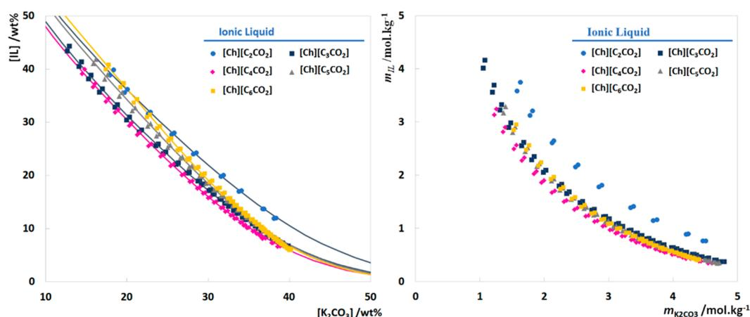
**Figure 2.** Orthogonal phase diagram representation for the ABS formed by IL +  $K_2CO_3$  + water at  $(298 \pm 1)$  K and atmospheric pressure. The solid lines represent the fitting by eq 1.
