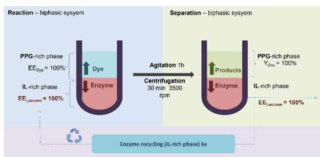
Figure 12 – Process developed using ABS as liquid supports for enzymatic degradation of dyes and enzyme reuse. Adapted from Ferreira *et al.* [188].
