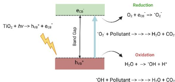
Figure 1 – Photocatalytic oxidation of organic compounds from textile wastewater under UV-TiO<sub>2</sub>. Adapted from Almamun *et al.* [72].
