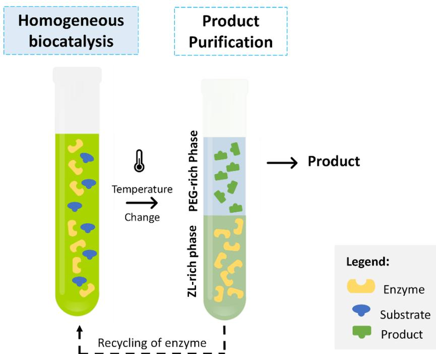
Figure 9. Flowchart of the integrated reaction-separation process developed, including the enzyme and ZI-rich phase recyclability. Adapted from Ferreira *et al.* [87].
