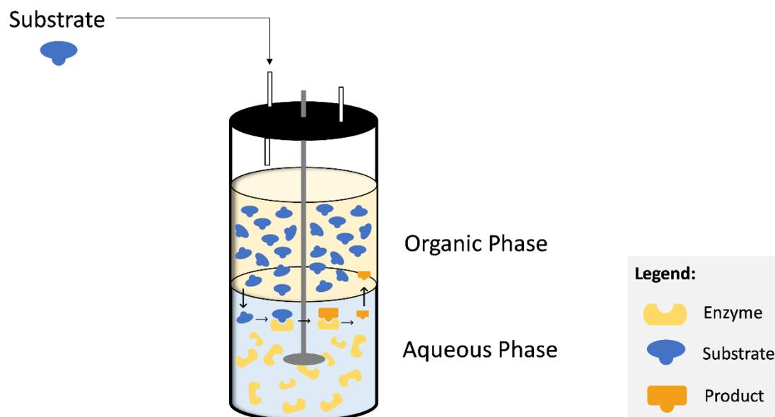
Figure 2. General scheme for two-phase partitioning bioreactors (TPPB) concept.
