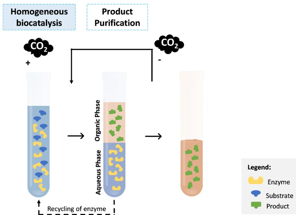
**Figure 3.** A proposed organic–aqueous tunable solvent (OATS) process for biocatalyst reuse. Adapted from Broering *et al.* [29].
