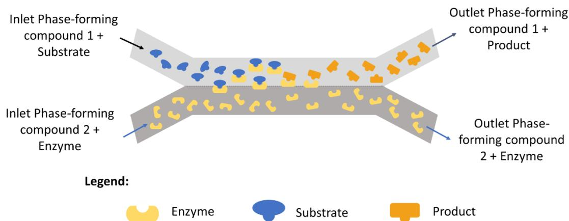
Figure 7. General scheme of an ABS microfluidic device for enzymatic reaction and product separation.
