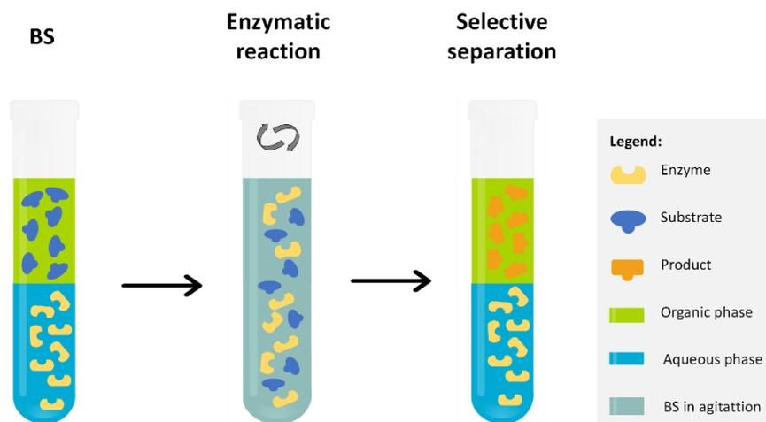
Figure 1. Schematic representation of a biocatalytic reaction in a heterogeneous medium using BS.
