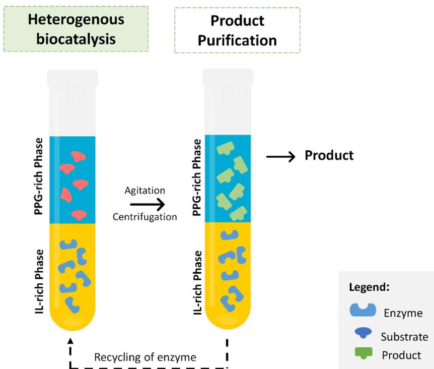
**Figure 8.** Integrated process using IL-based ABS for dye decolorization and enzyme reuse. Adapted from Ferreira *et al.* [61].
