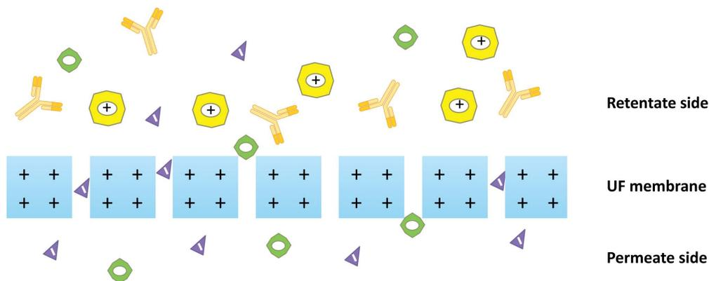
**Fig. (9).** Schematic representation of HPTFF process illustrated for the specific case of antibody purification using positively charged ultrafiltration (UF) membranes.
