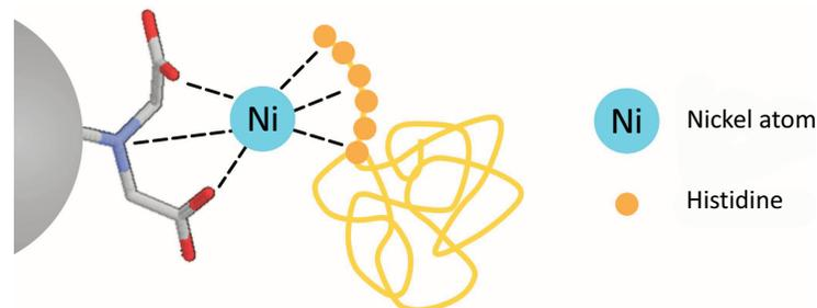
**Fig. (7).** Schematic representation of the interaction mechanism in immobilized metal affinity chromatography. The tridentate chelating agent IDA (iminodiacetic acid) coordinates with the nickel atom, which also interacts with the histidine tail present in the protein.
