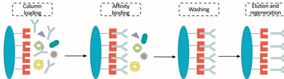
**Fig. (5).** Schematic representation of the mAbs capture step by protein A affinity chromatography.
