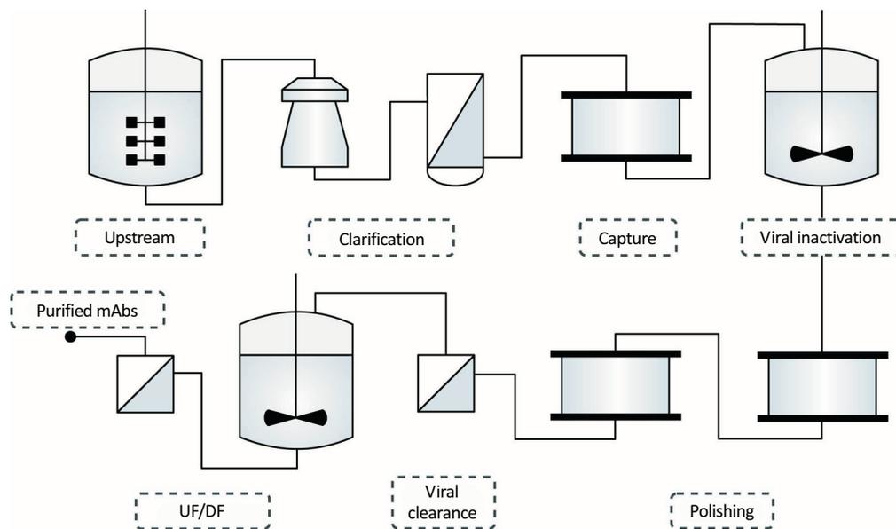
Fig. (4). Standard downstream platform for the purification of mAbs.
