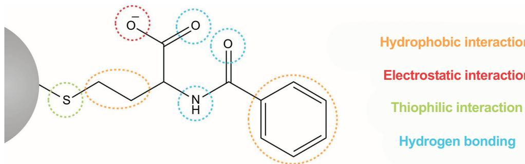
**Fig. (6).** Molecular structure of a multimodal ligand commercialized for monoclonal antibodies purification (Capto™ MMC), evidencing the several interactions that could be integrated.
