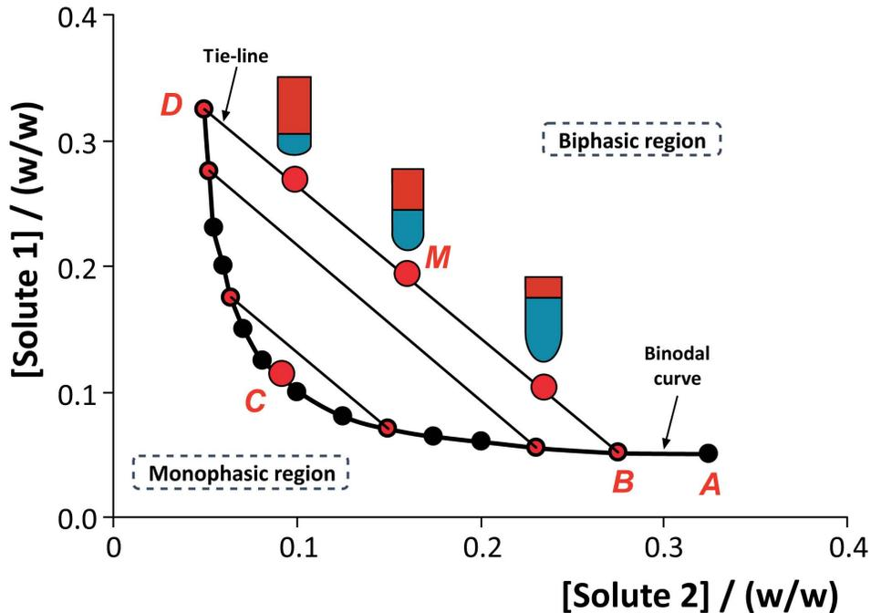
**Fig. (10).** Schematic representation of a phase diagram of an ATPS composed of two different solutes, in weight fraction, and where the concentration of water is omitted.
