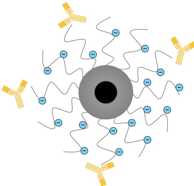
**Fig. (8).** Schematic representation of a magnetic separation process exemplifying the adsorption of antibodies on a modified magnetic nanoparticle with a negatively charged polymer.
