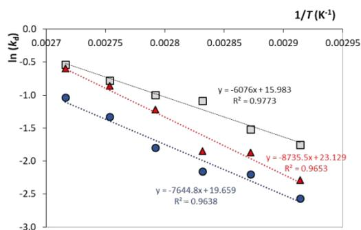
Semi-log plots of the first-order denaturation constant ( $k_d$ ) vs. the reciprocal temperature ( $1/T$ ). The slopes of the resulting straight lines were used to estimate the activation energies ( $E_d^*$ ) of irreversible inactivation (denaturation).
