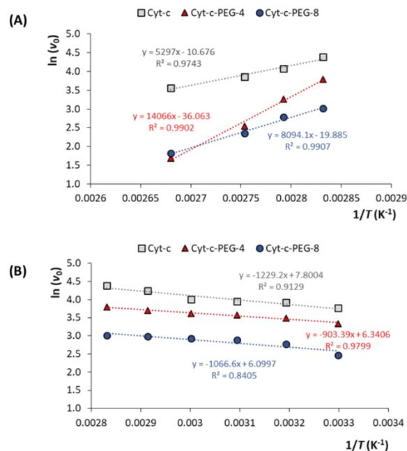
**Fig. 2.** Arrhenius-type plots of initial activity of Cyt-c and PEGylated conjugates with 4 (Cyt-c-PEG-4) or 8 (Cyt-c-PEG-8) PEGs attached, using 0.300 mM ABTS as a substrate. **(A)** temperature range 30–80°C ( $T < T_{\text{opt}}$ ) and **(B)** temperature range 80–100°C ( $T > T_{\text{opt}}$ ).
