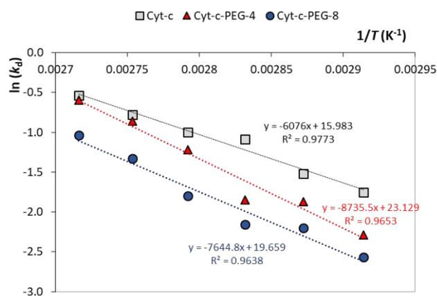
**Fig. 3.** Semi-log plots of the first-order denaturation constant ( $k_d$ ) vs. the reciprocal temperature ( $1/T$ ). The slopes of the resulting straight lines were used to estimate the activation energies ( $E^*_d$ ) of irreversible inactivation (denaturation) of native cytochrome c (Cyt-c) and PEGylated conjugated with 4 (Cyt-c-PEG-4) or 8 (Cyt-c-PEG-8) PEGs attached.
