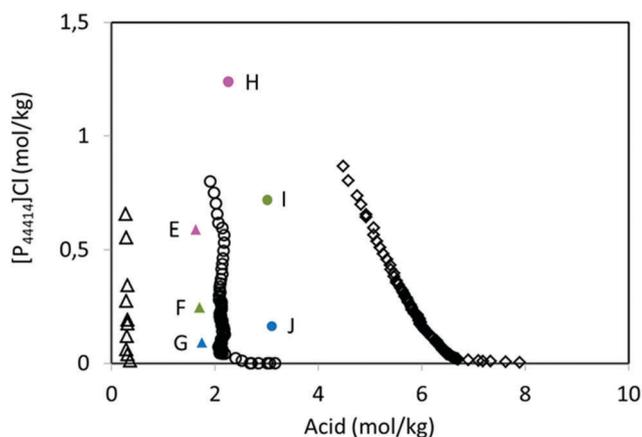
Fig. 4 Phase diagrams of AcABS composed of [P<sub>44414</sub>]Cl, water and the acids HCl (◊), H<sub>2</sub>SO<sub>4</sub> (○) and HNO<sub>3</sub> (△). The mixture points E, F and G belong to HNO<sub>3</sub>-based system and H, I and J to H<sub>2</sub>SO<sub>4</sub>-based system.
