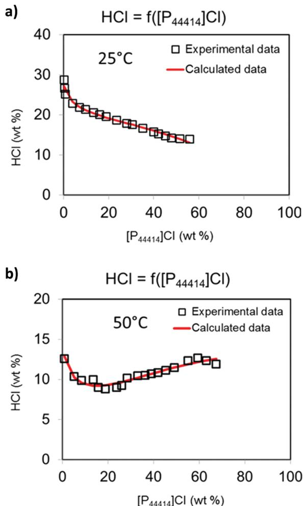
Fig. 2 Fitting of HCl-[P<sub>44414</sub>]Cl-H<sub>2</sub>O binodal curve experimental data at (a) 25 °C and (b) 50 °C for  $HCl = f([P_{44414}]Cl)$ .
