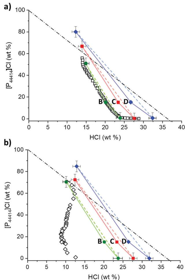
Fig. 3 Representation of the tie-lines for the ternary system HCl-[P<sub>44414</sub>]Cl-H<sub>2</sub>O at (a) 25 °C and (b) 50 °C.
