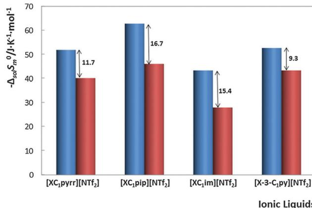
Fig. 3 Entropy of a solution of ILs for linear (blue bars) and branched alkyl chains (red bars) in water at 298.15 K.
