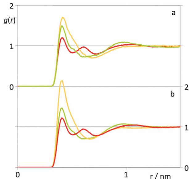
Fig. 7 Radial distribution functions in (a) pure ILs and in (b) IL mixtures with 0.3 water mole fraction, between the terminal carbon atoms of the alkyl chains, CT. Green =  $[C_3C_1im][NTf_2]$ , yellow =  $[C_4C_1im][NTf_2]$  and red =  $[i-C_4C_1im][NTf_2]$ .
