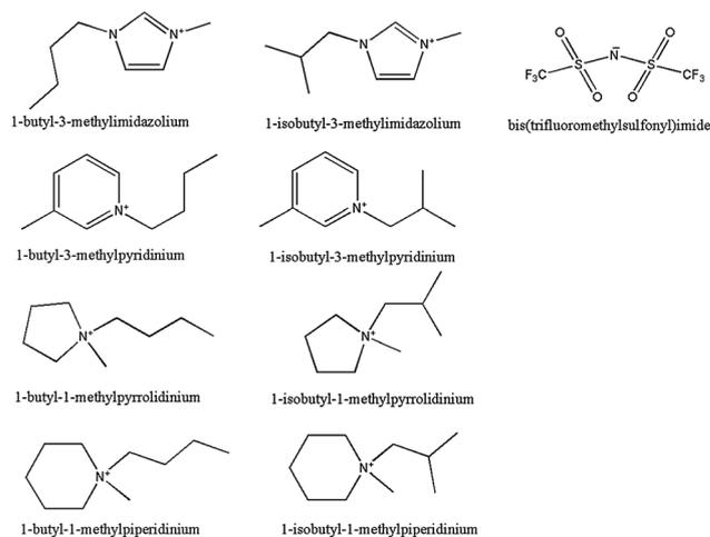
Fig. 1 Chemical structures of the ions constituting the ILs studied in this work.
