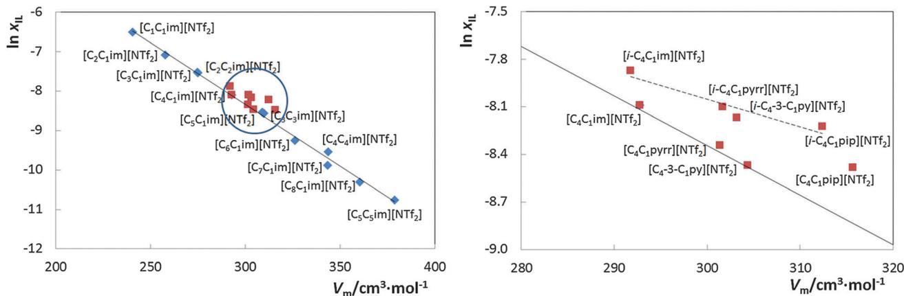
Fig. 4 Solubility of the studied ILs in water (expressed in mole fraction) as a function of the molar volume of ILs. All data are at 298.15 K. The solid lines represent the correlation between the ILs solubility in water and their molar volume taken from density data.<sup>44</sup> The dashed line is only presented to facilitate the interpretation.
