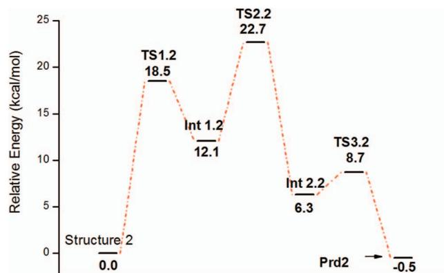
FIG. 14. Energy diagram associated with S-O exchange mechanism between CS<sub>2</sub> and acetate (with the Structure 2 as reference energy, Fig. 13) calculated for the system CS<sub>2</sub> + ion pair (IP) at the UB3LYP/6-31+(d,p):MQZVP(S) level. The calculated energy values associated with the (stationary points) transition states (TS), intermediate structures (Int), and final structures of the adducts (Prd2) along the reactive pathway are given in kcal/mol.
