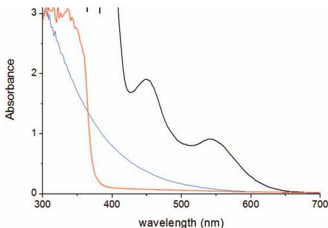
FIG. 8. UV-Visible spectrum of the  $\text{CS}_2$ -[BmPyrro] [Ac] solution ( $x_{\text{CS}_2} = 0.04$ ) compared with those of pure  $\text{CS}_2$  (red) and [BmPyrro] [Ac] (blue). The spectrum of the solution (black) has been recorded 30 min after preparation.
