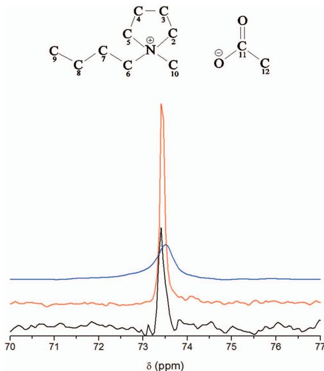
FIG. 2. <sup>15</sup>N NMR spectra of CS<sub>2</sub>-[BmPyrro] [Ac] solutions (*x*<sub>CS<sub>2</sub></sub> = 0.05, red, *x*<sub>CS<sub>2</sub></sub> = 0.20, blue) and of pure [BmPyrro] [Ac] (black).
