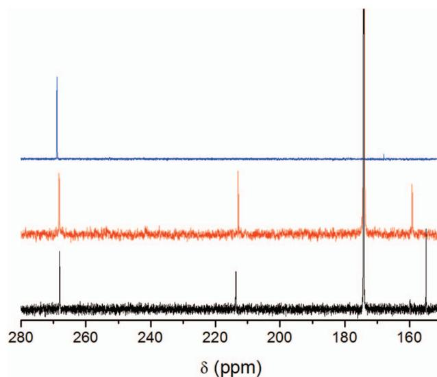
FIG. 6. Observation of the resonance line at about 269 ppm in the  $^{13}\text{C}$  NMR spectra of an aqueous solution of  $\text{Na}_2\text{CS}_3$  (0.07 mol  $\text{l}^{-1}$ , blue),  $\text{CS}_2$ -[BmPyrro][Ac] solution ( $x_{\text{CS}_2} = 0.05$ , red), and  $\text{CS}_2$ -[Bmim][Ac] solution ( $x_{\text{CS}_2} = 0.05$ , black).
