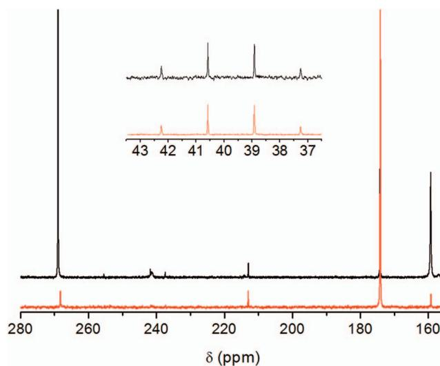
FIG. 5. Effect of the isotopic substitution of the carbon atom of  $\text{CS}_2$  in the  $^{13}\text{C}$  NMR spectra of  $\text{CS}_2$ -[BmPyrro][Ac] solutions ( $x_{\text{CS}_2} = 0.05$ ):  $\text{CS}_2$  (red), labeled  $^{13}\text{CS}_2$  (black). The inset shows a magnification of the spectra in the domain centered at about 40 ppm.
