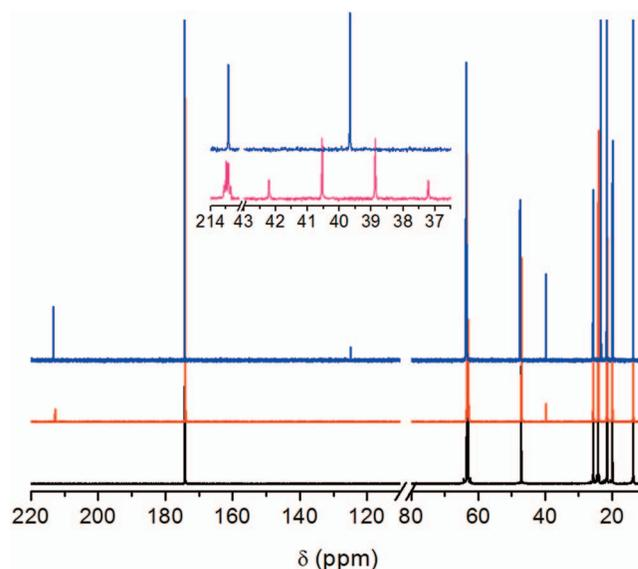
FIG. 3. Proton decoupled  $^{13}\text{C}$  NMR spectra of  $\text{CS}_2$ -[BmPyrro] [Ac] solutions ( $x_{\text{CS}_2} = 0.05$ , red,  $x_{\text{CS}_2} = 0.20$ , blue) and of pure [BmPyrro] [Ac] (black). The inset shows a magnification of the spectra (with and without proton decoupling) of the new resonance line (about 40 ppm) of the concentrated solution.
