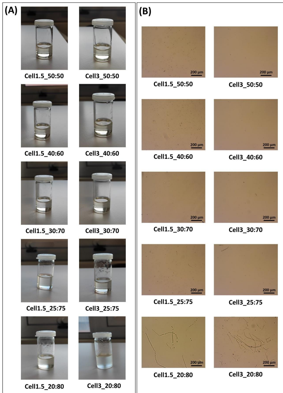
Fig. S1. (A) Digital photographs and (B) optical micrographs of the various cellulose solutions (1.5% and 3.0%, w/w) using different mass ratios of [Emim][OAc]:DMSO (50:50, 40:60, 30:70, 25:75 and 20:80).
