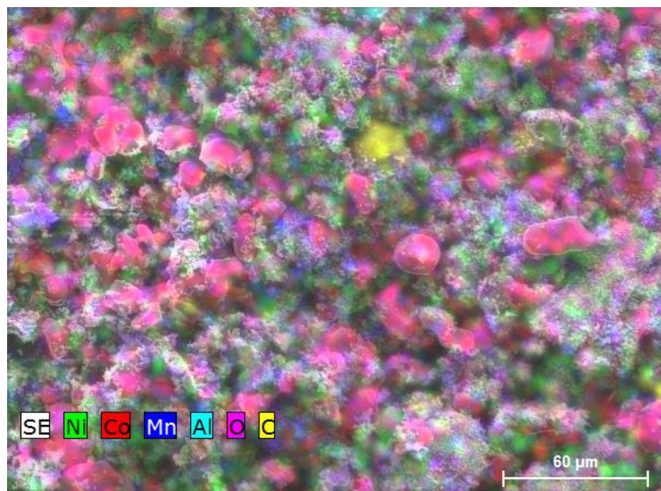
Figure S1. SEM-EDS of the black mass from spent cathode materials.
