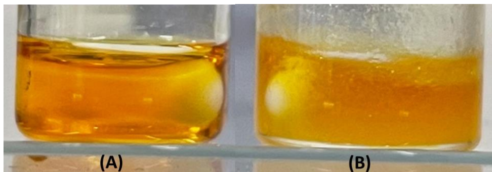
Fig. S4. Photo of IL solution with (A) 1.1 wt% K_2CO_3 and (B) 4.6 wt% K_2CO_3 after cellulose dissolution. Condition: 85 wt% [mTBNH][OAc], 7.5 wt% water and 7.5 wt% cellulose at 353.2 K for 24 hours.
