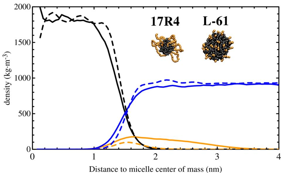
**Figure S4.** Micelle density profile comparison of 17R4 (solid) and L-61 (dashed) at 1 wt% of Pluronic concentration at the cloud point temperatures 38°C and 20°C, respectively. The color code is the same as in **Figure S3**.
