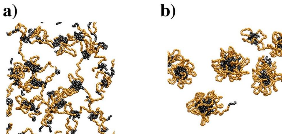
**Figure S7.** An example of initial stages (a) and later stages (b) of 10R5 micelle formation obtained in the MD simulations at 1 wt%. In a), isolated 10R5 moieties connect neighboring micelles in the initial micelle formation. In b), the PPG segments belonging to the micelle point outwards from the micelle core and can join the PPG core of close neighbor micelles.
