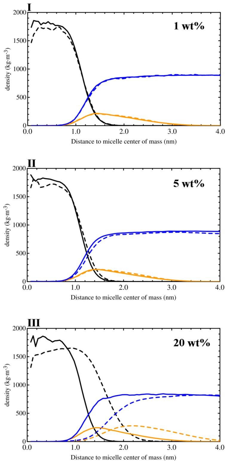
**Figure S6.** Density profile of 10R5 (dashed lines) and L-35 (solid lines) micelles at (I) 1, (II) 5 and (III) 20 wt% Pluronic concentration. The color code is the same as in **Figure S3**.
