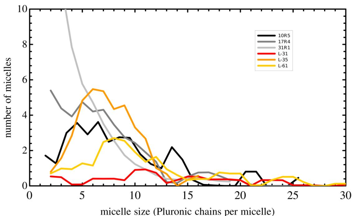
**Figure S2.** Micelle distribution for all Pluronics obtained with the cluster counting code. The micelle size distribution shows that the averaged micelle size distribution fall in the range of 5 to 15 Pluronic chains *per* micelle. Thus, the micelle distribution was divided in three groups with the most representative micelle size distribution group around 8 chains *per* micelle.
