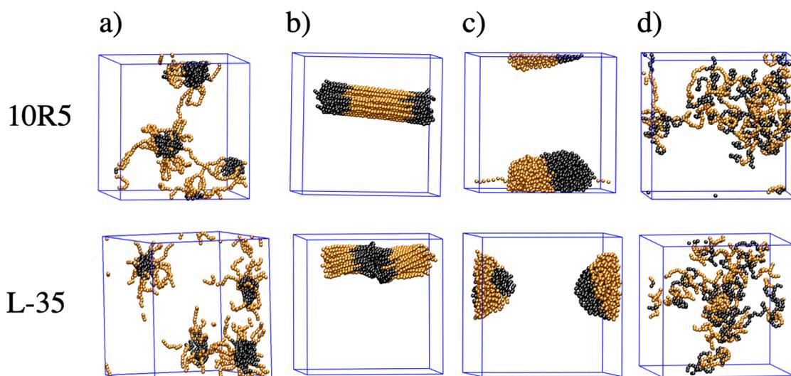
**Figure S1.** MD simulation snapshots after 1  $\mu$ s of simulations time for 10R5 (top) and L-35 (bottom). a) the model developed in this work, b) Hezaveh,<sup>1</sup> c) Hakateyama<sup>2</sup> and d) Nawaz.<sup>3,4</sup>
