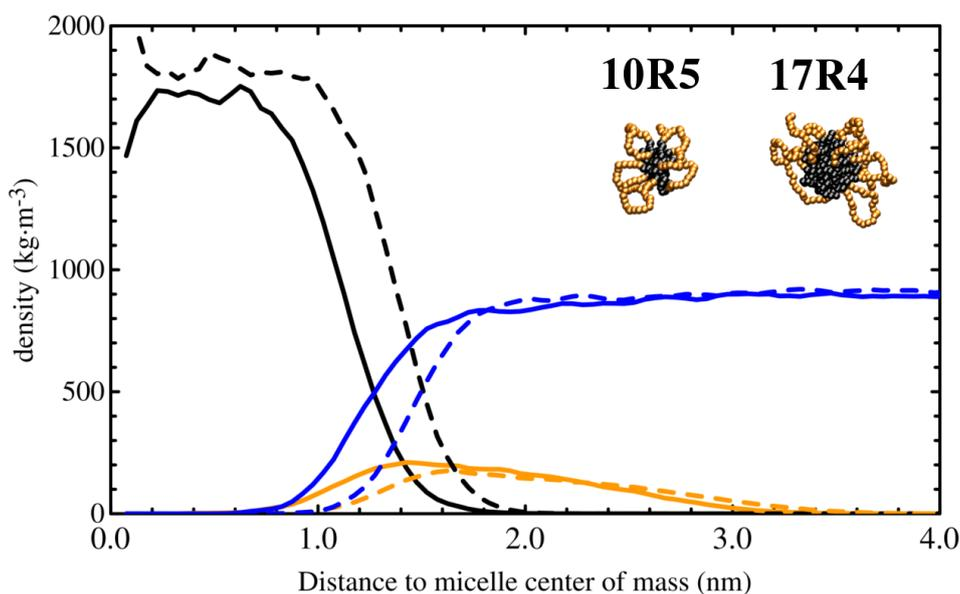
**Figure S3.** Micelle density profile comparison of 10R5 (solid) and 17R4 (dashed) at 1 wt% of Pluronic concentration at the cloud point temperatures 61°C and 38°C, respectively. The color code is PPG in black, PEG in orange and water in blue.
