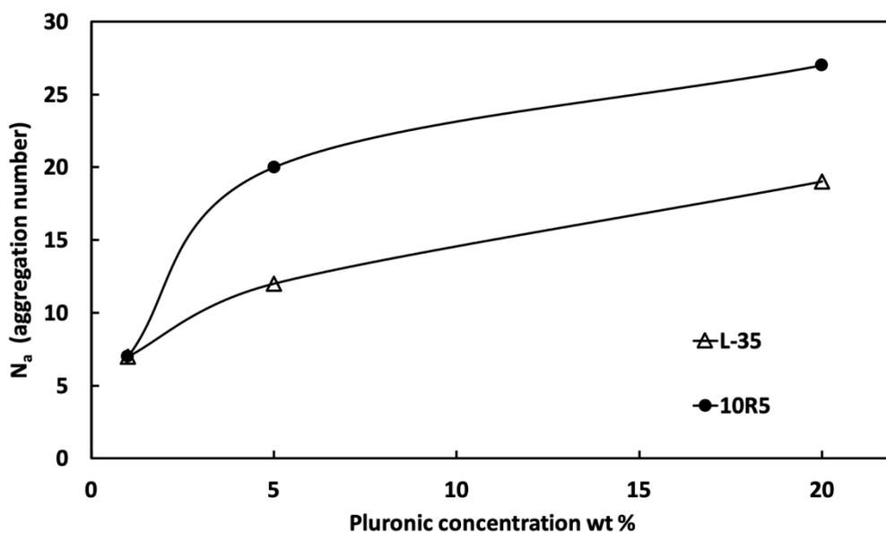
**Figure S5.** Aggregation number ( $N_a$ ) of L-35 ( $\Delta$ ) and 10R5 ( $\bullet$ ) micelles for 1, 5 and 20 wt% of Pluronic concentration at the cloud point temperatures shown in **Figure 10.II**.
