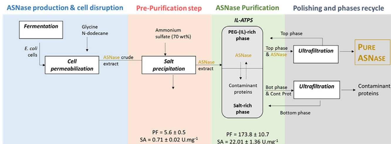
**Figure 9.** Schematic representation of the *in situ* purification process of periplasmic ASNase using polymer-based ATPS with  $[C_4mim][CH_3SO_3]$  as adjuvant. The isolation of ASNase and the recycling of both aqueous phases are also represented.
