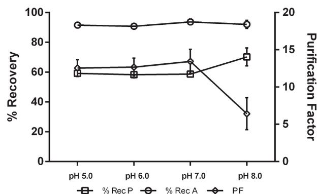
**Figure 2.** Recovery yield of total proteins (%Rec P) and ASNase (%Rec A), and purification factor of ASNase (PF) for the ATPS composed of PEG 6000 + citrate buffer (15 wt%/15 wt%) at different pHs. Error bars correspond to standard deviations obtained from three replicates.
