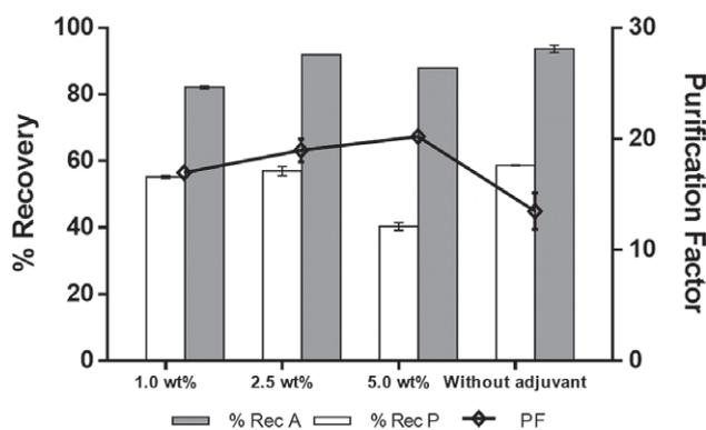
**Figure 6.** Recovery yield of total proteins (%Rec P) and ASANase (%Rec A) and purification factor (PF) in the ATPS composed PEG of 6000 + citrate buffer (15 wt%/15 wt%) at pH = 7 and with [C<sub>4</sub>mim][CH<sub>3</sub>SO<sub>3</sub>] as adjuvant. Errors bars correspond to standard deviations obtained from three replicates.
