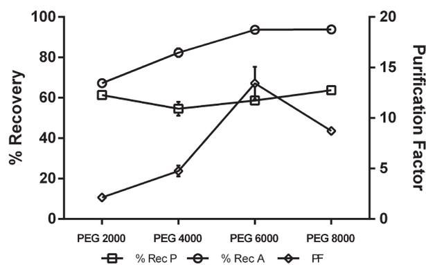
**Figure 1.** Recovery yield of total proteins (%Rec P) and ASNase (%Rec A) and purification factor of ASNase (PF) for the ATPS composed of PEG + citrate buffer (15 wt%/15 wt%) at pH 7. Errors bars correspond to standard deviations obtained from three replicates.
