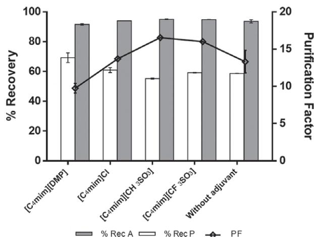
**Figure 5.** Recovery yield of total proteins (%Rec P) and ASANase (%Rec A), and purification factor (PF) in the ATPS composed of PEG 6000 + citrate buffer (15 wt%/15 wt%) at pH = 7 and with 1 wt% of [C<sub>4</sub>mim]-based ILs as adjuvants. Error bars correspond to standard deviations obtained from three replicates.
