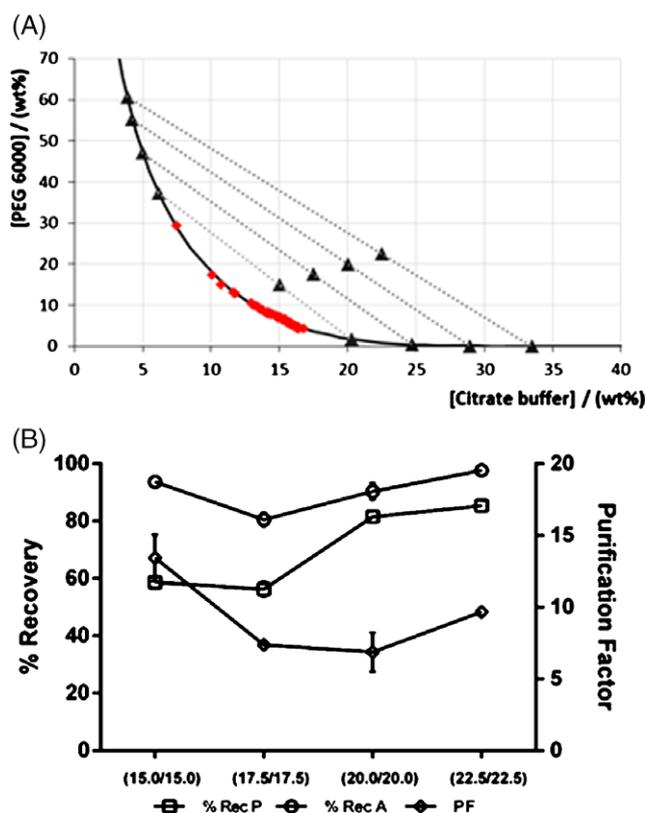
**Figure 4.** (A) Ternary phase diagram of PEG 6000 + citrate buffer system at pH = 7 with representation of tie-lines (TL) for the following mixture points: PEG 6000 wt%/citrate buffer wt% = 15.0/15.0; 17.5/17.5; 20.0/20.0; 22.5/22.5. (B) Recovery yields of total proteins (%Rec P) and ASNase (%Rec A) and purification factor (PF) for the PEG 6000 + citrate buffer ATPS at pH = 7, considering four distinct mixture points. Error bars correspond to standard deviations obtained from three replicates.
