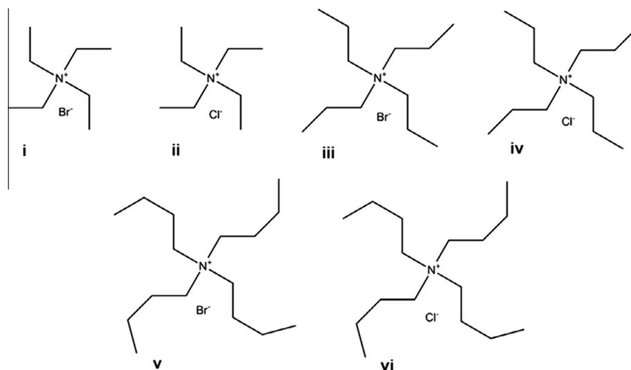
**Fig. 2.** Chemical structure of the ammonium compounds studied in this work:  $[N_{2,2,2,2}]Br$  (i),  $[N_{2,2,2,2}]Cl$  (ii),  $[N_{3,3,3,3}]Br$  (iii),  $[N_{3,3,3,3}]Cl$  (iv),  $[N_{4,4,4,4}]Br$  (v) and  $[N_{4,4,4,4}]Cl$  (vi).
