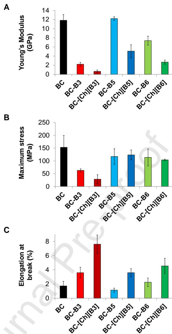
**Fig. 5.** Young's modulus (A), maximum stress (B) and elongation at break (C) of BC, BC-VIT and BC-[Ch][VIT] membranes.
