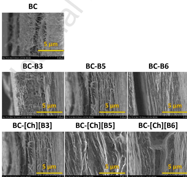
**Fig. 4.** SEM images of BC, BC-VIT and BC-[Ch][VIT] cross sections at  $\times 10k$  magnification.
