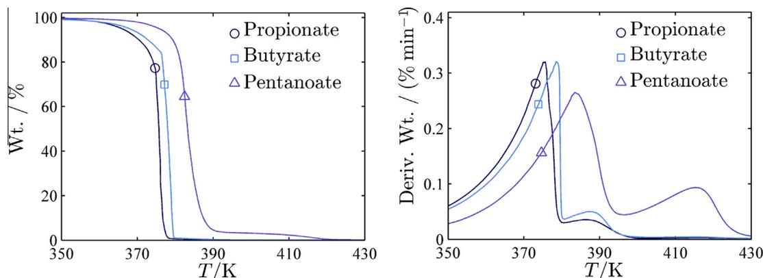
FIGURE 7. Thermogravimetric curves (left) and respective time derivatives (right) of the N-methyl-2-hydroxyethylammonium IL samples by HRMTGA (amplitude of modulation:  $\pm 5$  K; period of modulation 200 s) at  $2 \text{ K} \cdot \text{min}^{-1}$ .
