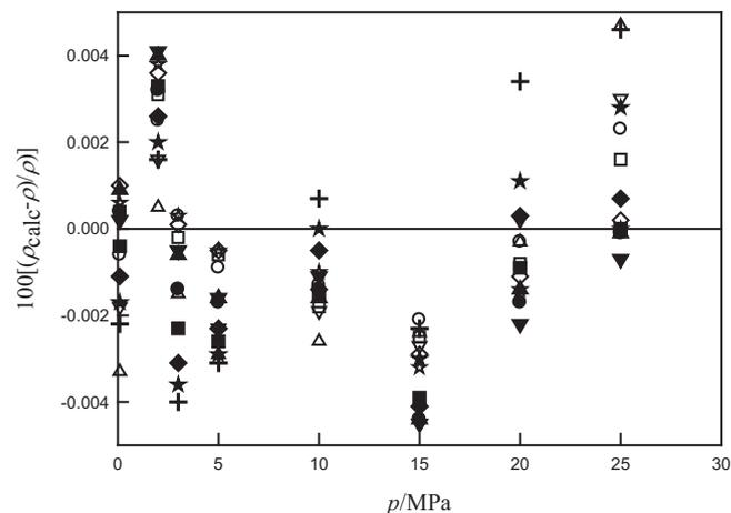
**FIGURE 5.** Relative density deviations between the calculated values with GMA EoS ( $\rho_{\text{calc}}$ ) and the experimental values ( $\rho$ ) for  $[\text{C}_2\text{OHC}_1\text{NH}_2][\text{C}_2\text{COO}]$ . Legend as in figure 2(a).
