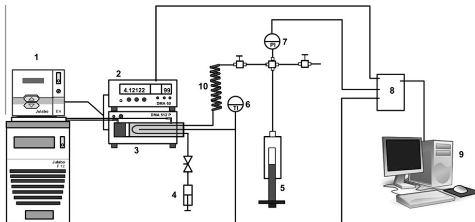
**FIGURE 1.** Experimental setup for the measurement of liquid densities at high pressures: 1, Julabo FP-50 thermostatic bath; 2, DMA 60 (Anton Paar) device for measuring the period of oscillation; 3, measuring cell DMA 512 P (Anton Paar); 4, syringe for sample introduction; 5, pressure generator model HIP 50-6-15; 6, PT probe; 7, pressure transducer Wika, S-10; 8, NI PCI-8220 data acquisition board; 9, PC; 10, buffer.
