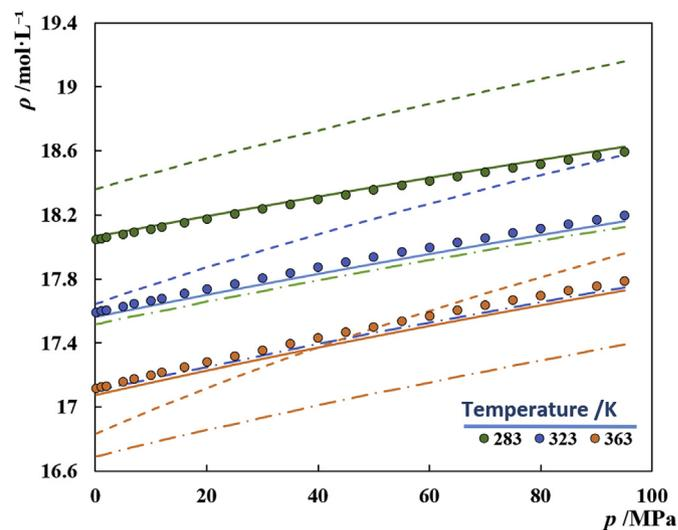
Fig. 1. High-pressure liquid densities of pure EG. Symbols represent experimental data [69] while the solid, dashed and long-dash-dotted lines represent the PC-SAFT predictions using the parameters proposed by Atilhan and Aparicio [86], Reschke et al. [87] and Liang et al. [88].
