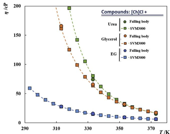
Fig. 5. Viscosities at 0.1 MPa for [Ch]Cl-based DES measured in this work. Circles represent the experimental data measured using the falling body viscometer while the squares with dashed lines represent the data measured using the SVM3000 device.
