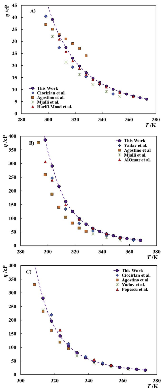
**Fig. 6.** Viscosities of [Ch]Cl-based DES with different HBDs: A) EG; B) glycerol and C) urea. Symbols represent literature data [36,42–47,51] while the circles with dashed lines depict the data measured in this work.
