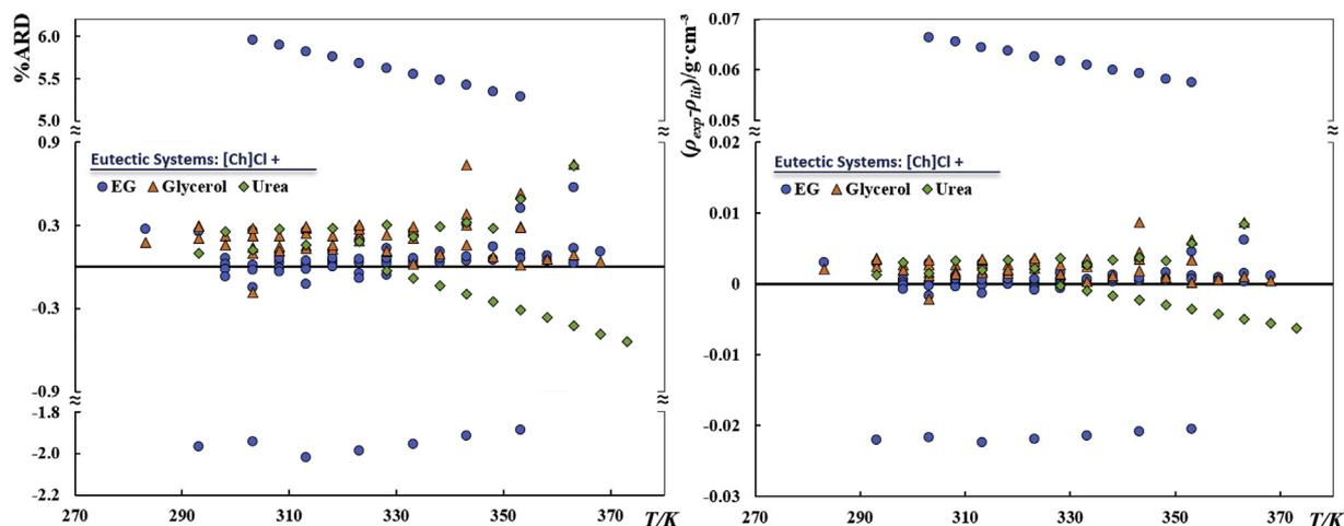
Fig. 2. Percentage average relative deviations (%ARD) (left) and density differences (right) between density data at atmospheric pressure measured in this work and those reported in literature [36–47]
