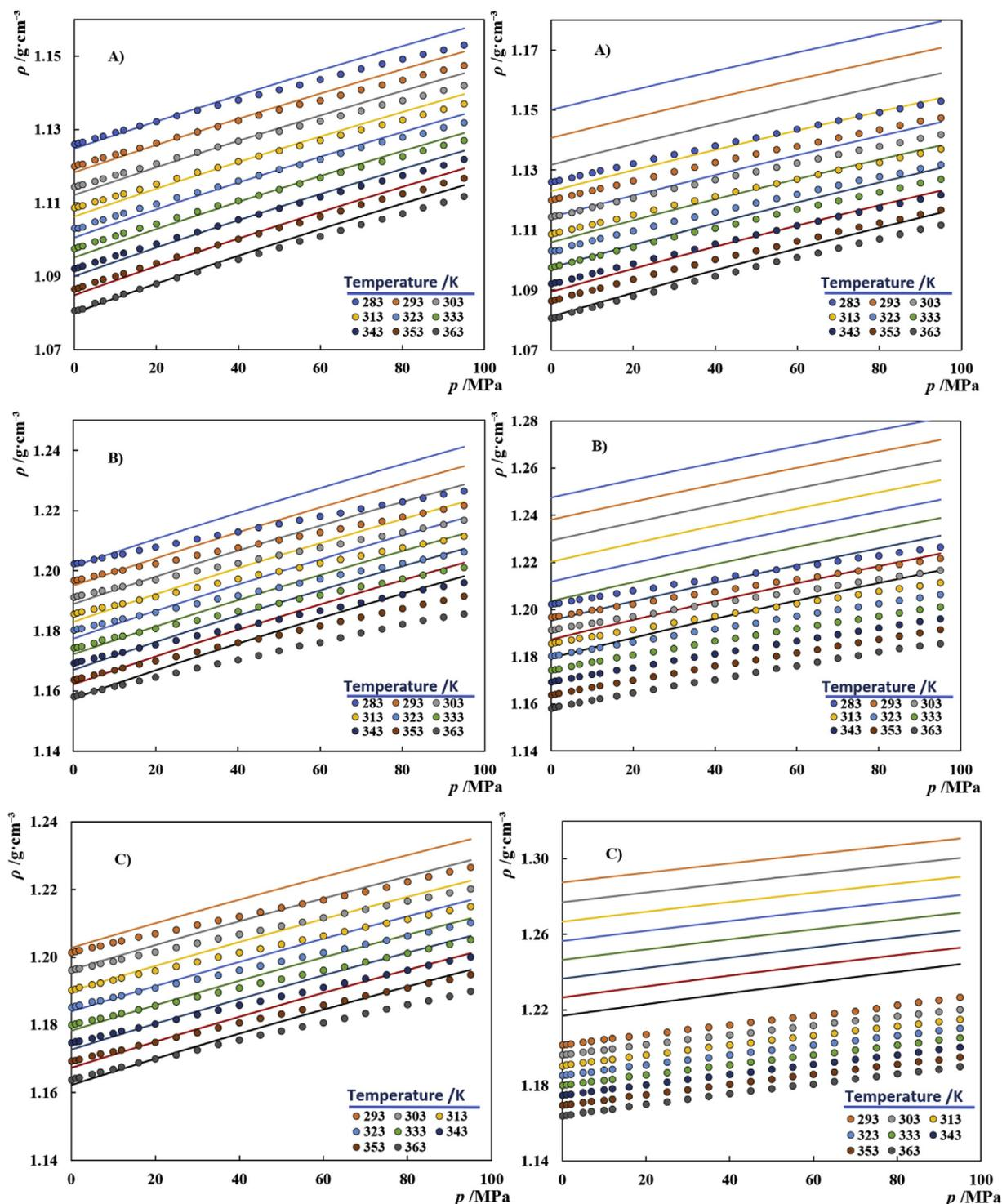
**Fig. 4.** High-pressure densities of [Ch]Cl-based DES with A) ethylene glycol B) glycerol C) urea as hydrogen bond donor. Symbols represent the experimental data measured in this work while the solid lines depict the PC-SAFT correlation of the data using a temperature-dependent binary interaction parameter (left) or the PC-SAFT predictions ( $k_{ij} = 0$ ) of the data (right).
