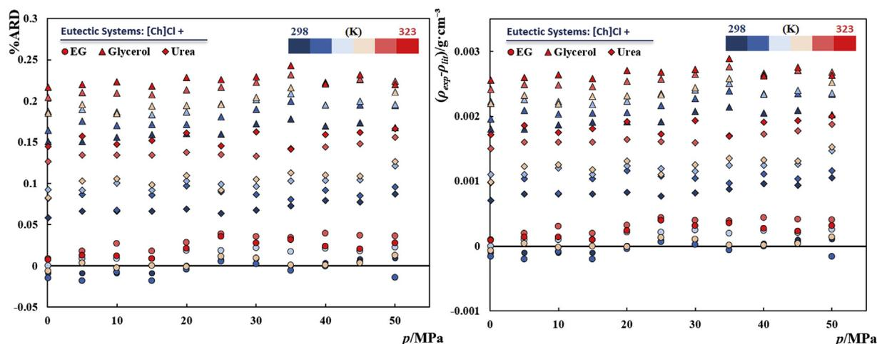
Fig. 3. Percentage average relative deviations (%ARD) (left) and density differences (right) between density data at pressures up to 50 MPa measured in this work and those reported in literature [48–50].
