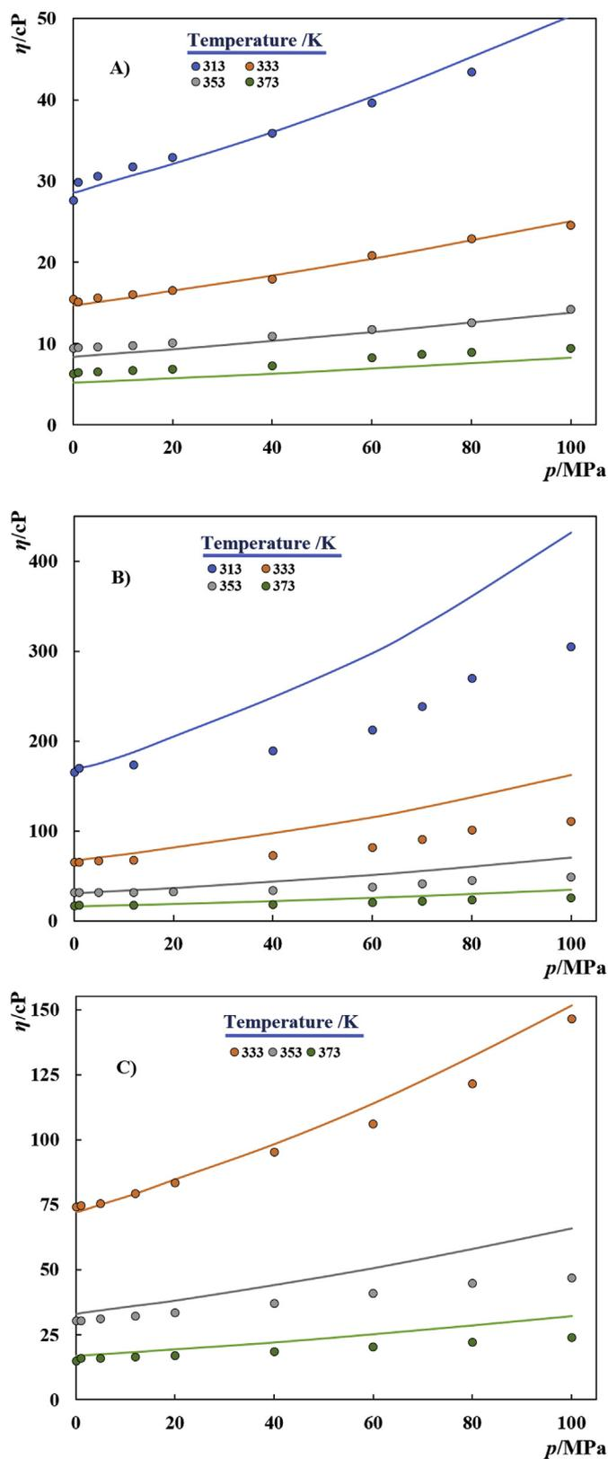
Fig. 7. Viscosities of [Ch]Cl-based DES with different HBDs. A) EG; B) Glycerol; C) Urea. Symbols represent experimental data measured in this work while the solid lines depict the results obtained with PC-SAFT + FVT.
