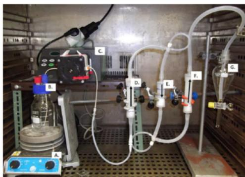
**Fig. 1.** Experimental setup for the continuous-regime experiment. A — stirring device; B — Feed mixture; C — Pump for reactional mixture feeding; D — 1st fixed bed bioreactor; E — Resin column; F — 2nd fixed bed bioreactor; G — Sampling point.
