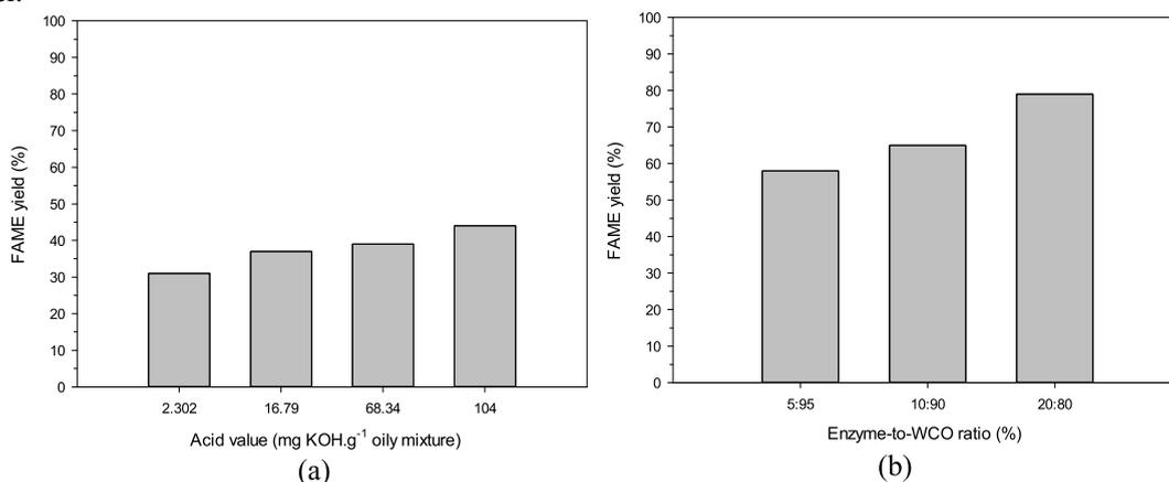
**Fig. 2.** FAME yield as function of (a) acidity, from different oily mixtures; and (b) enzyme-to-WCO ratio. Conditions: 50 °C, 8 h, MeOH/oily mixture = 4:1 (mol/mol), acid value of 104 mg KOH g<sup>-1</sup>.
