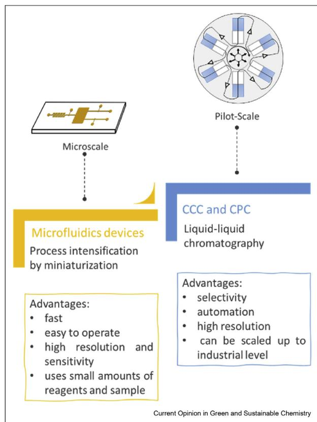
Schematic illustration of microfluidics and CPC/CCC devices and related advantages. CPC, centrifugal partition chromatography; CCC, counter-current chromatography.
