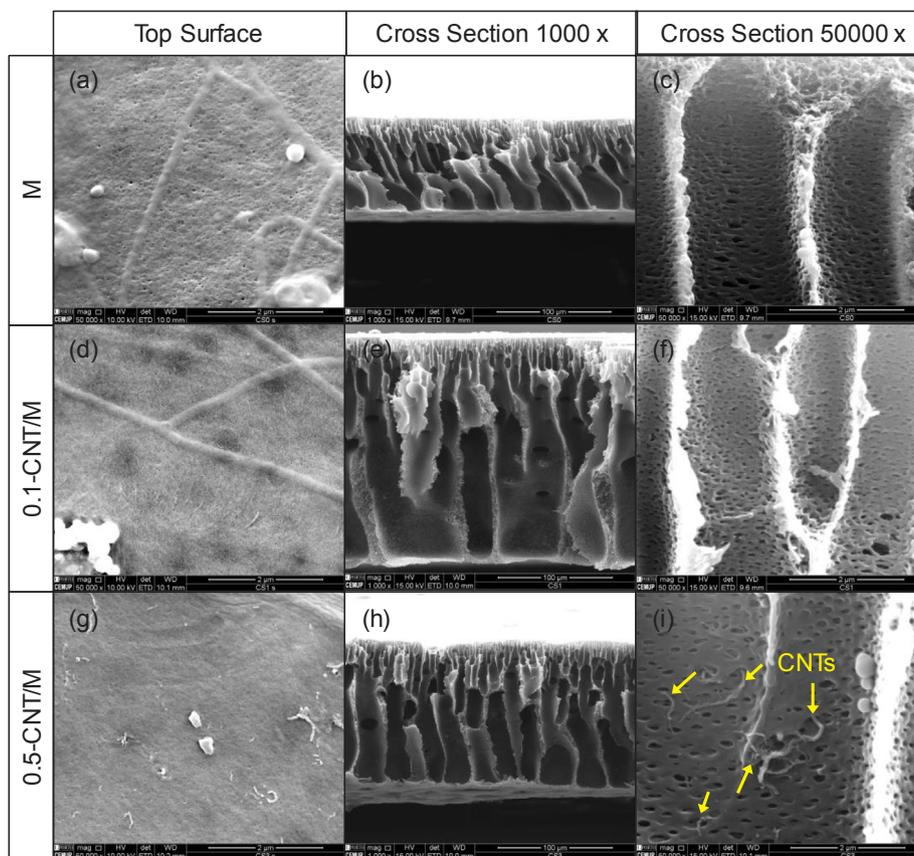
Fig. 2. SEM images of the (a, d and g) top surface and (b-c, e-f, and h-i) cross-section of the neat PSf membrane (a-c) and functionalized CNT/M membranes (d-i).
