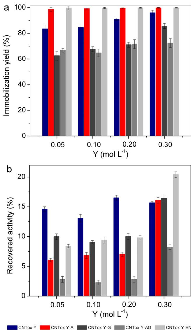
**Fig. 3.** Laccase immobilization efficiency (a), and recovered activity (b), as a function of  $\text{HNO}_3$  concentration (Y) for surface modified CNTs. Experimental conditions: laccase immobilized in 50 mM phosphate buffer (pH 8.0) under orbital stirring for 2 h at 25 °C.
