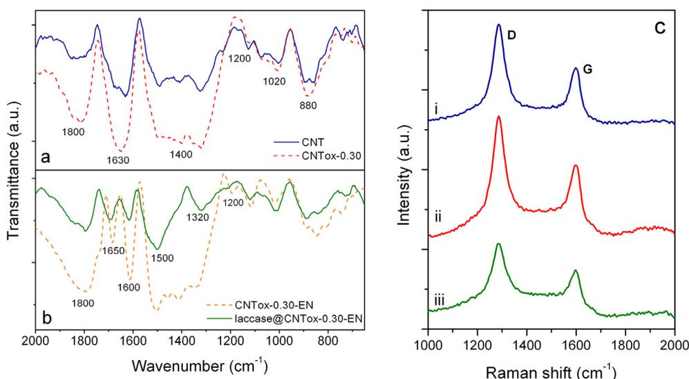
Fig. 1. FTIR-ATR spectra of: (a) CNT and CNTox-0.30; (b) CNTox-0.30-EN and laccase immobilized on CNTox-0.30-EN. (c) Raman spectra of pristine CNT (i), CNTox-0.30-EN (ii) and laccase immobilized on CNTox-0.30-EN (iii).
