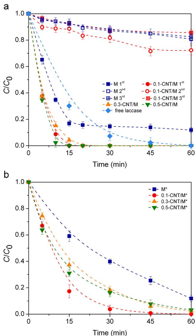
**Fig. 7.** (a) Degradation of MP using laccase immobilized over the different PSf membranes, the 2nd and 3rd utilizations for M and 0.1-CNT/M are also included for comparison; (b) degradation of MP using a second immobilization of laccase on used PSf membranes (M\*). Experimental conditions: reactions using 20 mL of 10 mg L<sup>-1</sup> MP aqueous solutions at natural pH (5.6).
