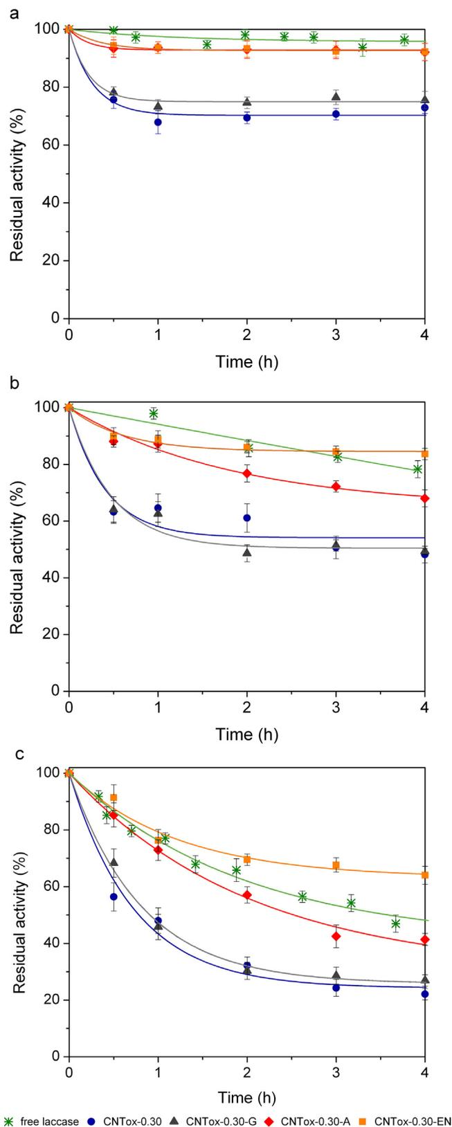
Fig. 4. Thermal inactivation of free and immobilized laccase, measured in terms of residual activity (%) over a period of 4 h, in phosphate buffer (100 mM, pH 8.0) at temperatures of: (a) 40 °C; (b) 50 °C; and (c) 60 °C.
