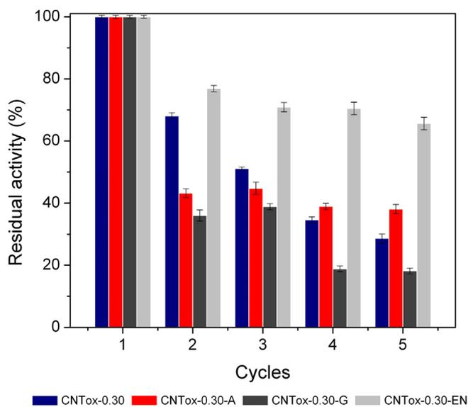
**Fig. 5.** Residual immobilized laccase activity in 5 consecutive cycles of catalytic reaction. Experimental conditions: laccase immobilized in 50 mM phosphate buffer (pH 8.0) under orbital stirring for 2 h at 25 °C.
