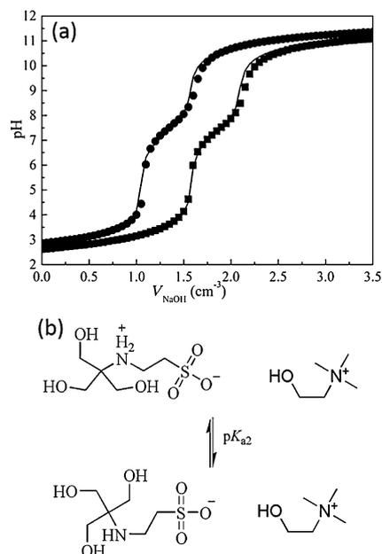
**Figure 1.** (a) pH titration curves of  $1 \times 10^{-3}$  M TES (■) and [Ch][TES] (●) at 25.0 °C and  $I = 0.1$  M of  $\text{NaNO}_3$ . (b) Protonation equilibrium of [Ch][TES].
