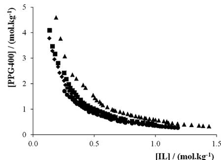
**Figure 2.** Ternary phase diagrams for the systems composed of PPG 400 + GB-IL + water at 25 °C and atmospheric pressure: [Ch][MES] (triangles), [Ch][Tricine] (diamonds), [Ch][TES] (squares) and [Ch][HEPES] (circles).
