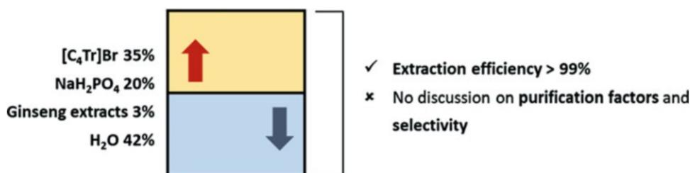
**Application of Ionic Liquids in Separation and Fractionation Processes, Fig. 12** Overview of the process proposed by He et al. [78] for the extraction of ginseng saponins
