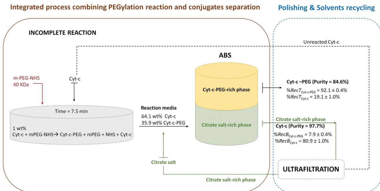
Fig. 5 Schematic diagram of the integrated process combining the bioconjugation reaction and separation with the polishing step and solvent recycling process for an incomplete PEGylation reaction. The dashed line represents steps that were not experimentally developed.
