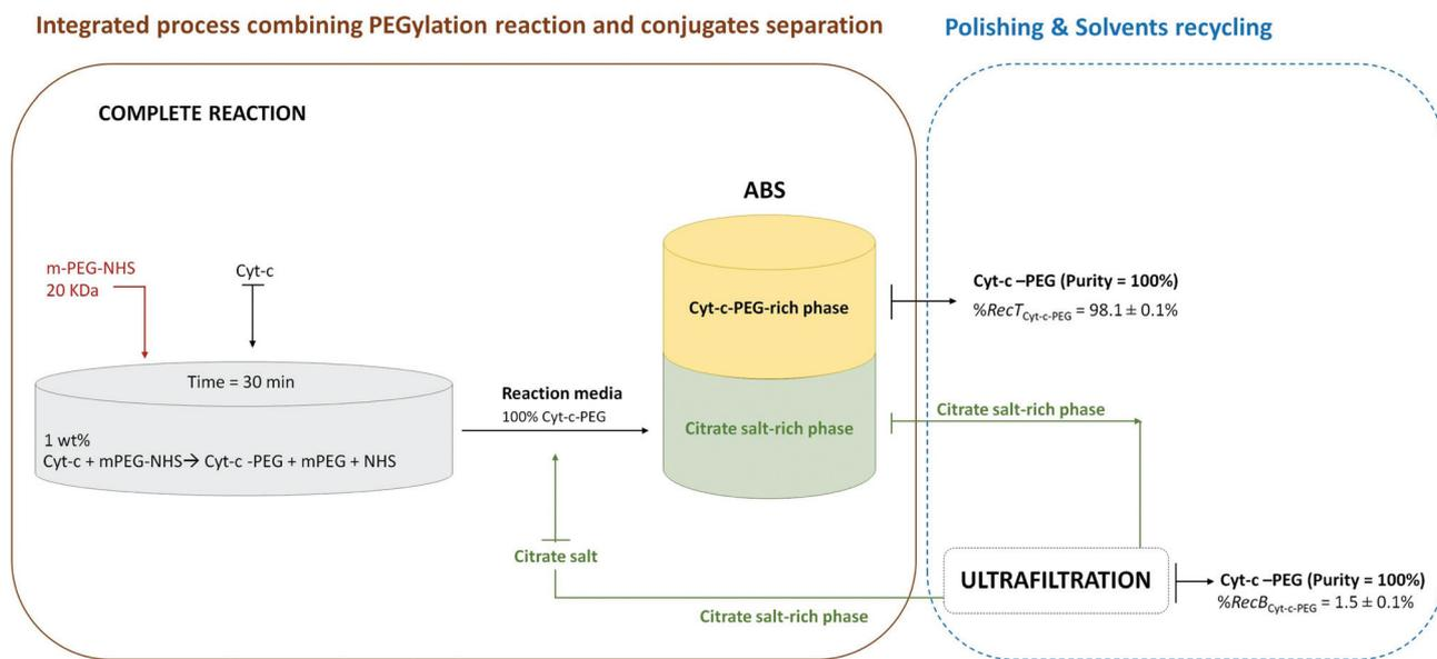
Fig. 4 Schematic diagram of the integrated process combining the bioconjugation reaction and separation with the polishing step and solvent recycling process for a complete PEGylation reaction. The dashed line represents steps that were not experimentally developed.
