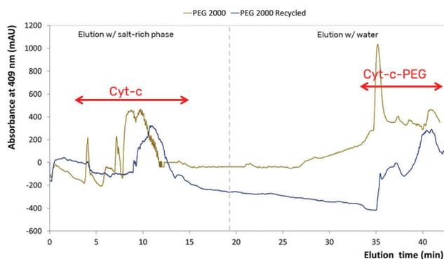
**Fig. 3** Chromatogram of fast centrifugal partition chromatography (FCPC) representing the separation of unreacted Cyt-c and Cyt-c-PEG, obtained after two-steps of PEGylation + fractionation using FCPC and the ABS comprising 15 wt% of PEG 2000 + 20 wt% of potassium phosphate buffer at pH 7.0.
