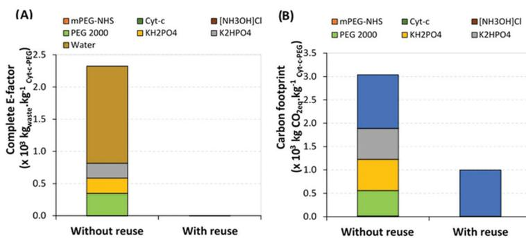
Fig. 4 Complete E-factor (A) and carbon footprint (B) of the integrated process to purify Cyt-c-PEG, for both scenarios explored, with and without the reuse of Cyt-c, PEG 2000, KH<sub>2</sub>PO<sub>4</sub>, K<sub>2</sub>HPO<sub>4</sub>, and water.
