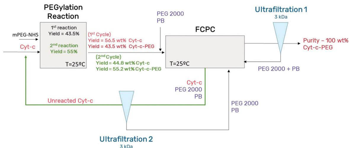
**Fig. 2** Process diagram of the integrated process of purification in a continuous regime applying fast centrifugal partition chromatography (FCPC) with PEG 2000 and phosphate buffer (PB), including the recycle of the unreacted Cyt-c and main solvents used.
