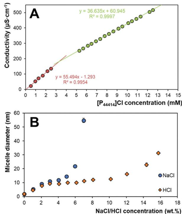
Fig. 4 (A) Variation in the conductivity of aqueous  $[P_{44414}]Cl$  solutions at 298 K as a function of  $[P_{44414}]Cl$  concentration. (B) Influence of NaCl and HCl concentrations on the  $[P_{44414}]^+$  micelle diameter in 20 wt%  $[P_{44414}]Cl$  solution at 298 K.
