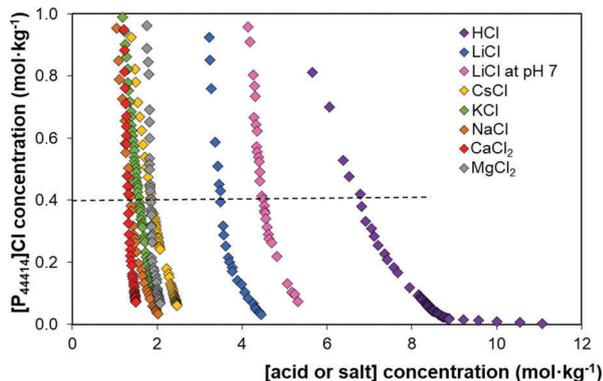
Fig. 3 Binodal curves for the ABS and AcABS composed of HCl, LiCl, NaCl, KCl, CsCl, MgCl<sub>2</sub> and CaCl<sub>2</sub> with [P<sub>44414</sub>]Cl at 298 K.
