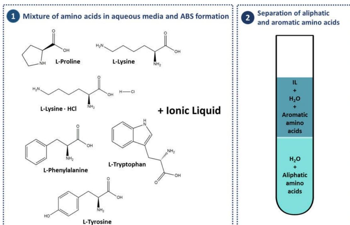
Figure 1. Chemical structures of the investigated amino acids and schematic view of the proposed process for the selective separation of aliphatic and aromatic amino acids mixtures.
