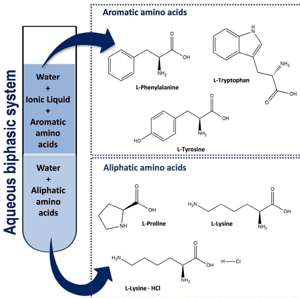
Ionic-liquid-based aqueous biphasic systems allow an efficient and selective separation of aliphatic and aromatic amino acids mixtures usually present in protein hydrolysates or fermentation broths
