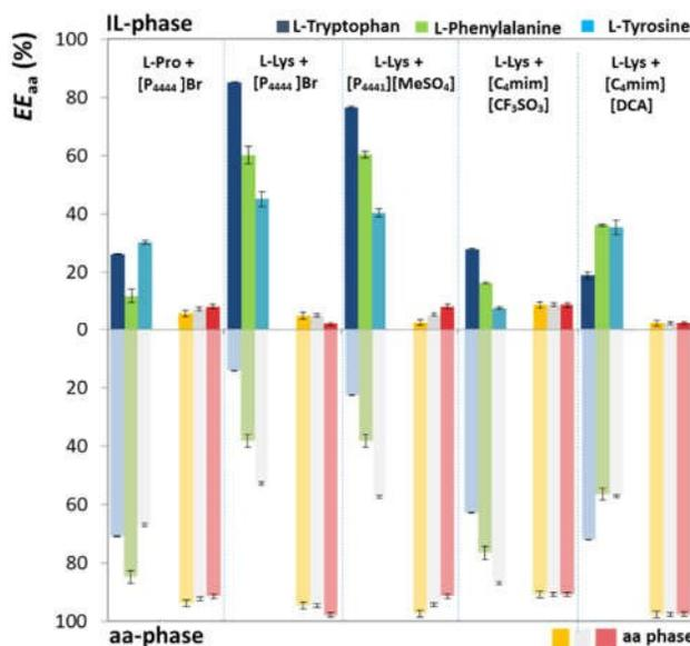
**Figure 3.** Extraction efficiencies of amino acids ( $EE_{aa}$ %) in the studied systems at 25°C. ■ ■ ■ represents the  $EE_{aa}$ % of aliphatic amino acids to the IL-rich opposite phase.
