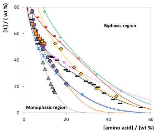
**Figure 2.** Phase diagrams of ABS composed of ILs + amino acids + H<sub>2</sub>O at 25°C: [P<sub>444(14)</sub>]Cl + L-Lys HCl (▲); [P<sub>4444</sub>]Br + L-Lys HCl (●); [N<sub>4444</sub>]Br + L-Lys HCl (■); [P<sub>4444</sub>]Br + L-Pro (◆); [P<sub>444(14)</sub>]Cl + L-Pro (—); [P<sub>4441</sub>][MeSO<sub>4</sub>] + L-Pro (+); [P<sub>444(14)</sub>]Cl + L-Lys (—); [P<sub>4444</sub>]Br + L-Lys (\*); [P<sub>4441</sub>][MeSO<sub>4</sub>] + L-Lys (×).
