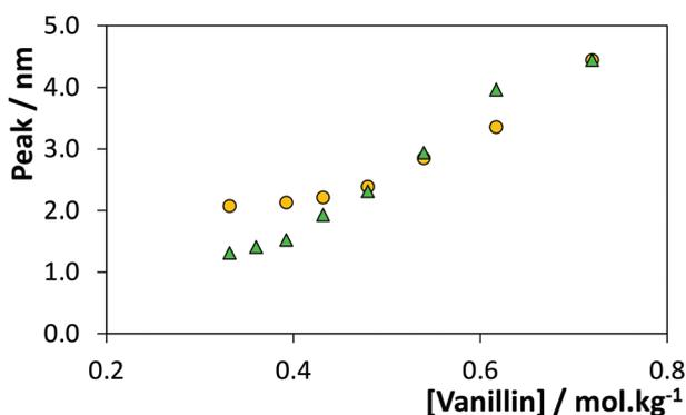
Fig. 10 Aggregate size change with the vanillin concentration: (●) constant hydrotrope concentration, *i.e.*, different vanillin/IL ratios, and (▲) constant ratio between the vanillin and hydrotrope concentrations.
