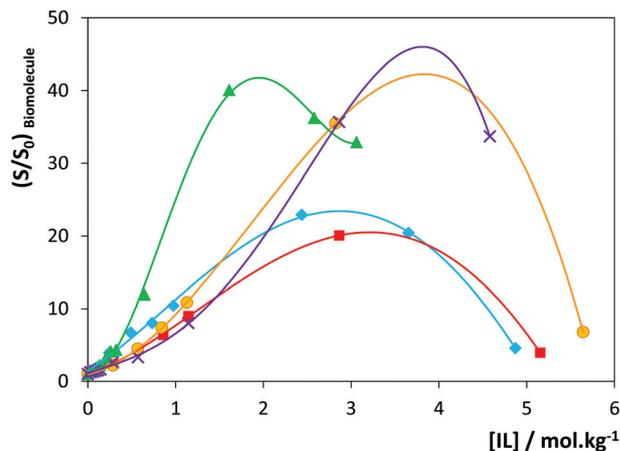
Fig. 3 Influence of the IL concentration on the solubility of gallic acid in aqueous solutions of (♦)  $[\text{C}_4\text{C}_1\text{im}][\text{N}(\text{CN})_2]$ , and (■)  $[\text{C}_4\text{C}_1\text{im}]\text{Cl}$ ; and vanillin in aqueous solutions of (●)  $[\text{C}_2\text{C}_1\text{im}][\text{N}(\text{CN})_2]$ , (▲)  $[\text{C}_4\text{C}_1\text{im}][\text{TOS}]$  and (×)  $[\text{C}_4\text{C}_1\text{im}]\text{Cl}$  at 303 K. Lines are guides for the eye.
