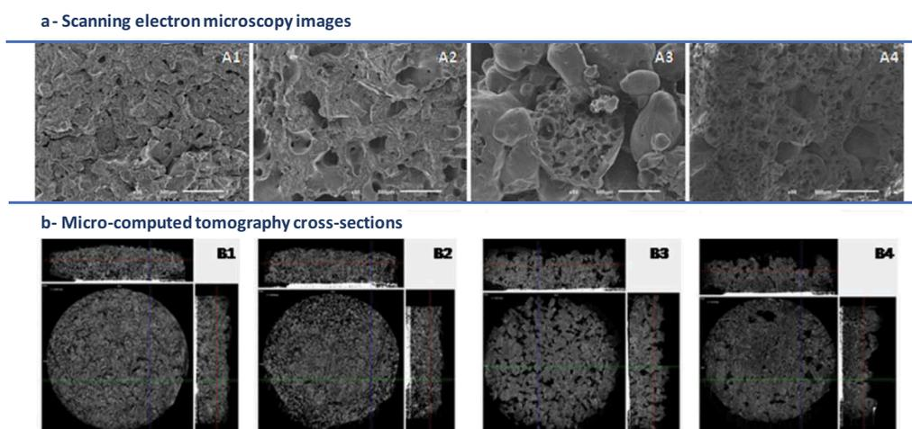
**Figure 4.** SEM images and micro-CT images of SPCL (B1), SPCL + ibuprofen (B2); SPCL + 10% API-DES (B3), and SPCL + 20% API-DES (B4) (Reproduced with permission from [44]).
