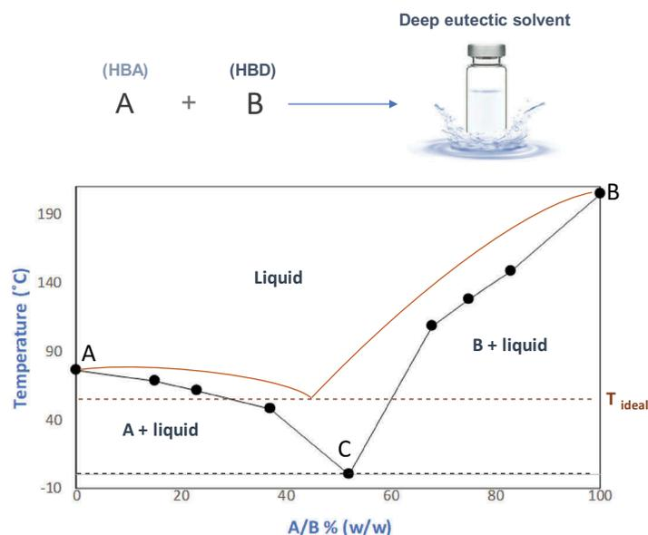
Figure 1. Phase diagram of a DES showing the depression of the freezing point of the mixture ( $T_E$ ) compared with its ideal behavior ( $T_{ideal}$ ).
