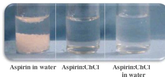
Figure 3. Visual representation of aspirin:ChCl liquid form using the API-DES strategy and subsequently improved solubility in water (Reproduced with permission from [45]).
