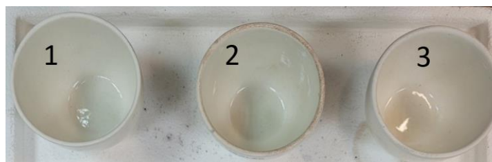
Figure S5. Beakers after biomass incineration following a single extraction cycle with [N_{4,4,4,4}]\text{Br} :hexanol (1:2). The starting biomass mass was approximately 2.81 g, and no residue was detected after incineration at 600 °C for 6 h, indicating that mineral extraction did not occur.
