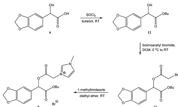
7 and 8 precipitated from the diethyl ether solution as white solids, with yields of 50% and 60%, respectively. In the case of IL 6, heating to reflux of the reaction mixture was required to ensure full conversion, with the final product 6 obtained as a white solid in 90% yield (Table 2). Overall yields for ILs 6–8 starting from 3,4-methylenedioxymandelic acid or 3,4-dimethoxymandelic acid are 6 58%, 7 38%, and 8 46%.
