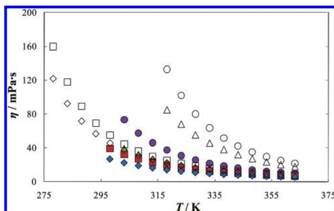
**Figure 5.** Experimental viscosity as a function of temperature, and at 0.1 MPa, for the dried ILs (empty symbols) and water-saturated ILs (full symbols):  $\diamond$ ,  $\blacklozenge$ , [C<sub>3</sub>mim][NTf<sub>2</sub>];<sup>56</sup>  $\square$ ,  $\blacksquare$ , [C<sub>3</sub>mpy][NTf<sub>2</sub>];<sup>57</sup>  $\Delta$ ,  $\blacktriangle$ , [C<sub>3</sub>mim][PF<sub>6</sub>];  $\circ$ ,  $\bullet$ , [C<sub>3</sub>mpy][PF<sub>6</sub>].
