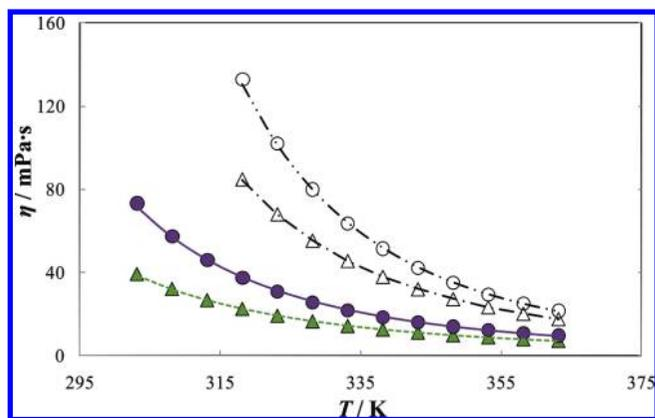
**Figure 6.** Experimental viscosity as a function of temperature, and at 0.1 MPa, for the dried ILs (empty symbols), water-saturated ILs (full symbols), and respective correlations using the Vogel–Tammann–Fulcher<sup>65</sup> method (lines):  $\Delta$ ,  $- \cdot -$ ,  $- - -$ , [C<sub>3</sub>mim][PF<sub>6</sub>];  $\circ$ ,  $- \cdot - \cdot -$ ,  $- -$ , [C<sub>3</sub>mpy][PF<sub>6</sub>].
