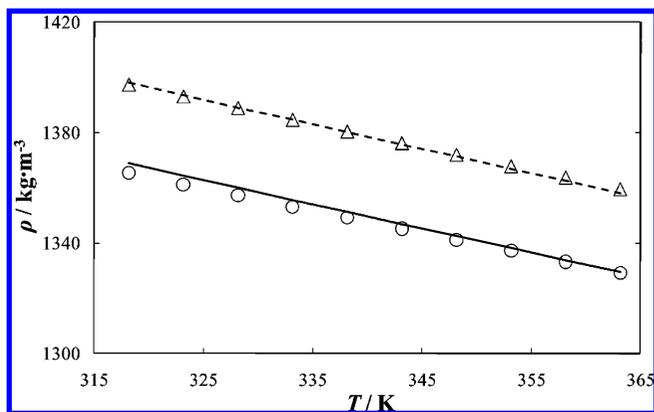
**Figure 4.** Experimental density as a function of temperature, and at 0.1 MPa, for the dried ILs (symbols) and respective prediction with the Gardas and Coutinho group contribution method<sup>45</sup> (lines):  $\Delta$ , ---, [C<sub>3</sub>mim][PF<sub>6</sub>];  $\circ$ , —, [C<sub>3</sub>mpy][PF<sub>6</sub>].
