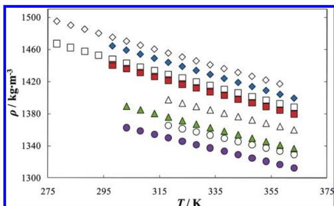
**Figure 3.** Experimental density as a function of temperature and at 0.1 MPa for the dried ILs (empty symbols) and water-saturated ILs (full symbols):  $\diamond$ ,  $\blacksquare$ , [C<sub>3</sub>mim][NTf<sub>2</sub>];<sup>56</sup>  $\square$ ,  $\blacksquare$ , [C<sub>3</sub>mpy][NTf<sub>2</sub>];<sup>57</sup>  $\triangle$ ,  $\blacktriangle$ , [C<sub>3</sub>mim][PF<sub>6</sub>];  $\circ$ ,  $\bullet$ , [C<sub>3</sub>mpy][PF<sub>6</sub>].
