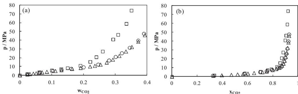
Fig. 7. Experimental solubility values (a) in mass fraction and (b) in mole fraction of the systems CO<sub>2</sub>+ castor oil (□), CO<sub>2</sub> + HOSO (Δ) and CO<sub>2</sub> + rapeseed oil (○) at 323 K.
