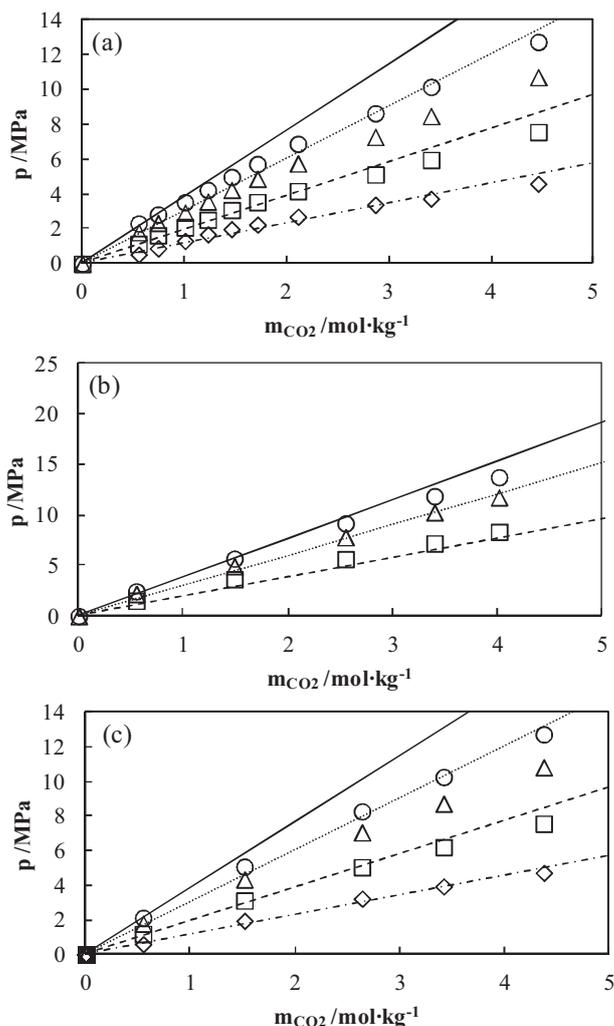
Fig. 8. Experimental solubility values of CO<sub>2</sub> in (a) HOSO, (b) castor oil and (c) rapeseed oil. Lines represent the Carvalho and Coutinho model [27]. 298 K (◇, ---), 323 K (□, - - -), 348 K (Δ, ...) and 363 K (○, -).
