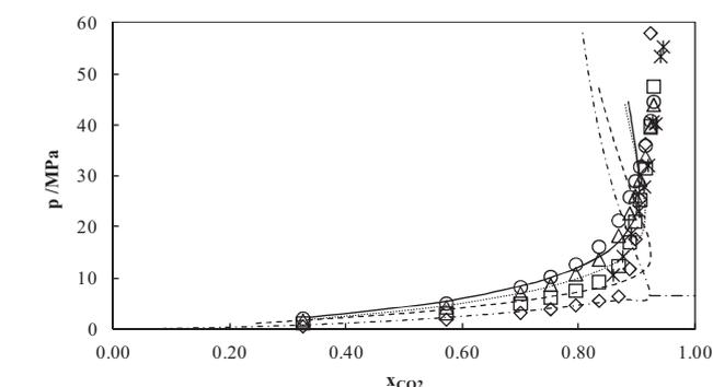
**Fig. 5.** Experimental solubility data of the system CO<sub>2</sub> + rapeseed oil at 298 K (◇), 323 K (□), 348 K (△) and 363 K (○). Data from Klein and Schulz [25] at 333 K (\*). Lines represent the SRK EoS with two interaction parameters ( $k_{ij}$  and  $l_{ij}$ ) from Table 8 at 298 K (---), 323 K (— · —), 348 K (···) and 363 K (— · · —).
