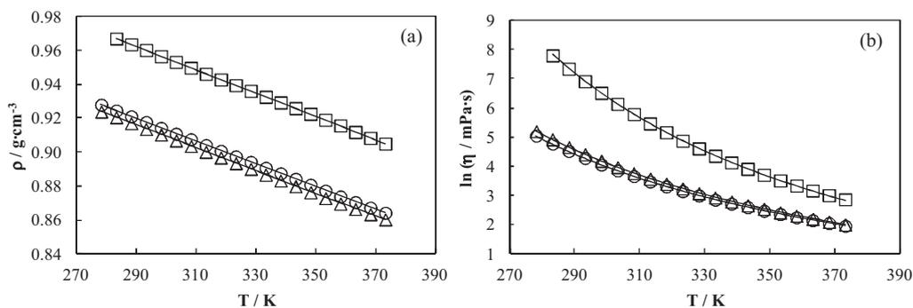
Fig. 1. (a) Experimental density and (b) viscosity values of the oils measured in this work. (□) Castor oil, (○) rapeseed oil and (△) HOSO. Lines represent correlations according to Eqs. (14) and (15) for density and viscosity values, respectively.
