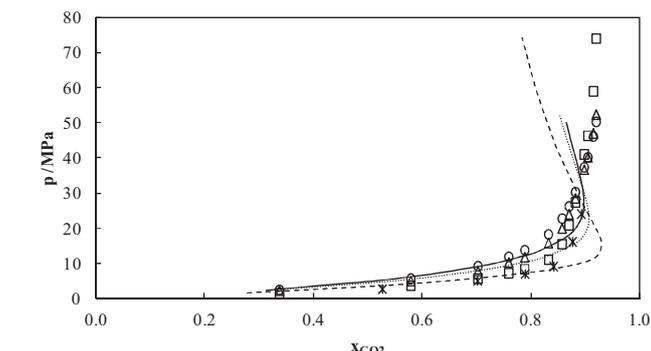
**Fig. 4.** Experimental solubility data of the system CO<sub>2</sub> + castor oil at 323 K (□), 348 K (△) and 363 K (○). Data from Ndiaye et al. [26] for the system CO<sub>2</sub> + castor oil at 323.15 K (\*). Lines represent the SRK EoS with two interaction parameters ( $k_{ij}$  and  $l_{ij}$ ) from Table 8 at 323 K (---), 348 K (···) and 363 K (—).
