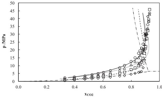
**Fig. 3.** Experimental solubility data of the system CO<sub>2</sub> + HOSO at 298 K (◇), 323 K (□), 348 K (△) and 363 K (○). Data from Fernández-Ronco et al. [47] for the system CO<sub>2</sub> + sunflower oil at 325.9 K (\*). Lines represent the SRK EoS with two interaction parameters (*k<sub>ij</sub>* and *l<sub>ij</sub>*) from Table 8 at 298 K (---), 323 K (—), 348 K (· · ·) and 363 K (—).
