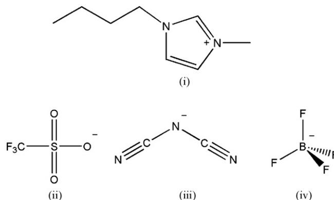
**Fig. 1.** Chemical structure of the cation and anions composing the ILs studied: (i) [C<sub>4</sub>mim]<sup>+</sup>; (ii) [CF<sub>3</sub>SO<sub>3</sub>]<sup>-</sup>; (iii) [N(CN)<sub>2</sub>]<sup>-</sup>; (iv) [BF<sub>4</sub>]<sup>-</sup>.
