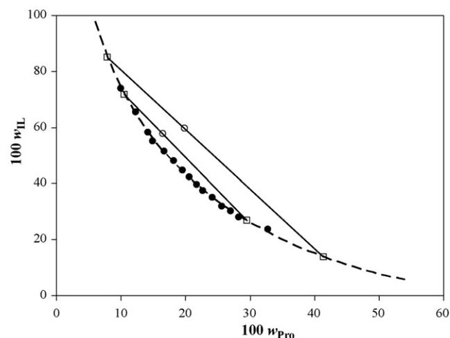
**Fig. 5.** Phase diagram for the [C<sub>4</sub>mim][CF<sub>3</sub>SO<sub>3</sub>]+Pro+water ternary system at 298 K: ●, binodal experimental data; ○, experimental data used for the TL determination; □, TL data; ---, fitting by Eq. (1).
