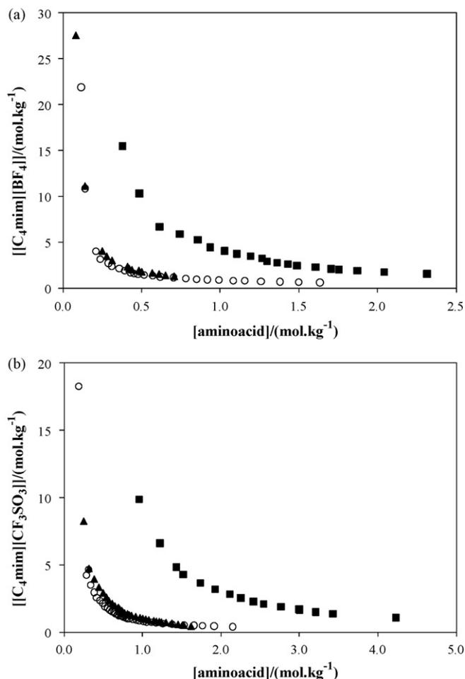
**Fig. 3.** Phase diagrams for the  $[C_4mim]$ -based ternary systems, at 298 K, composed by (a)  $[C_4mim][BF_4]$  + aminoacid +  $H_2O$ ; (b)  $[C_4mim][CF_3SO_3]$  + aminoacid +  $H_2O$ : ○, Lys; ▲, Lys-HCl; ■, Pro.
