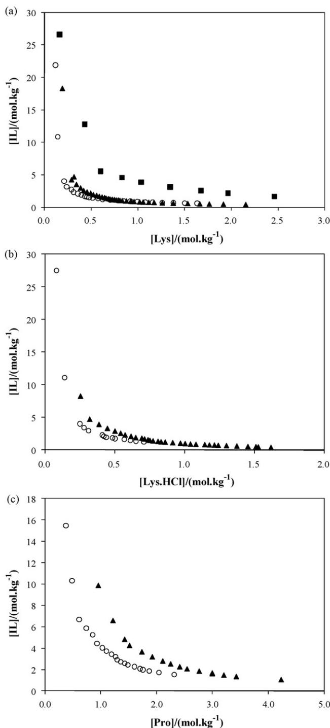
**Fig. 4.** Phase diagrams for the  $[C_4mim]$ -based ternary systems, at 298 K, composed by (a) IL + Lys +  $H_2O$ ; (b) IL + Lys-HCl +  $H_2O$ ; (c) IL + Pro +  $H_2O$ : ○,  $[C_4mim][BF_4]$ ; ▲,  $[C_4mim][CF_3SO_3]$ ; ■,  $[C_4mim][N(CN)_2]$ .
