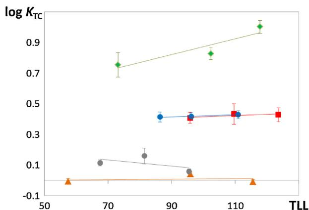
**Fig. 1.** Logarithm of  $K_{TC}$  versus TLL, at 25 °C, for the systems composed of PEG600+[Ch]-based salt+water: (◆) [Ch]Bic; (■) [Ch]Ac; (●) [Ch]DHph; (●) [Ch]DHcit; (▲) [Ch]Cl.
