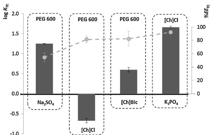
**Fig. 2.** Logarithm of K<sub>TC</sub> (■) and %EE<sub>TC</sub> (●) obtained in several ATPS formed with the fermented broth.
