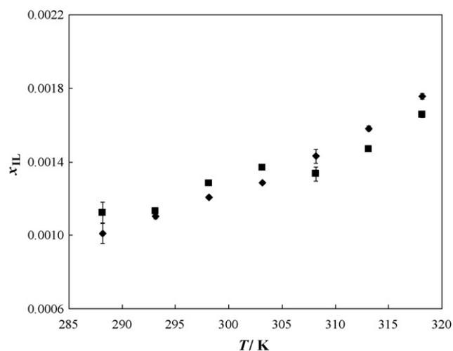
**Fig. 1.** Mole fraction solubility of  $[C_4mim][PF_6]$  in water as a function of temperature determined by (◆) UV-vis spectroscopy [9] and (■) ESI-MS (this work).
