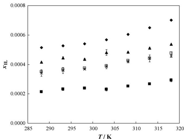
**Fig. 2.** Mole fraction solubility of ILs in water as a function of temperature: (◆)  $[C_3mim][Tf_2N]$  [11]; (▲)  $[C_3mpyr][Tf_2N]$ ; (□)  $[C_3mpy][Tf_2N]$  [9]; (×)  $[C_3mpip][Tf_2N]$ ; (■)  $[C_4mpyr][Tf_2N]$ .
