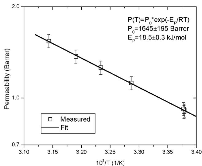
Fig. 5. Temperature dependence of  $\text{CO}_2$  permeability in PLA ( $L:D=98.7:1.3$ ).
