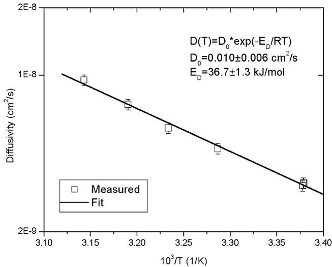
Fig. 6. Temperature dependence of CO<sub>2</sub> diffusivity in PLA ( $L:D=98.7:1.3$ ).
