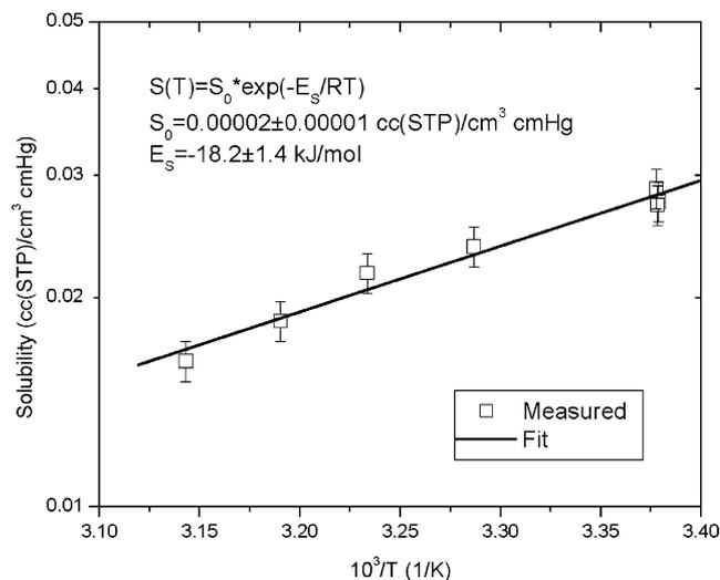
Fig. 7. Temperature dependence of CO<sub>2</sub> solubility in PLA ( $L:D=98.7:1.3$ ).
