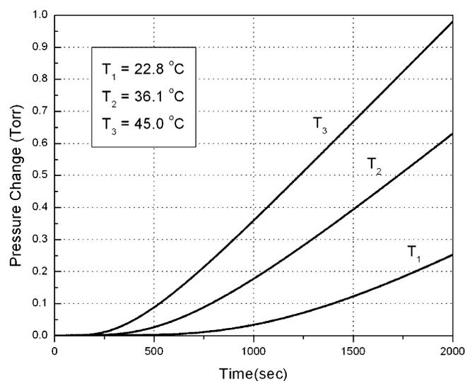
Fig. 4. Typical time lags for  $\text{CO}_2$  permeation in PLA ( $L:D=98.7:1.3$ ) under different temperatures.
