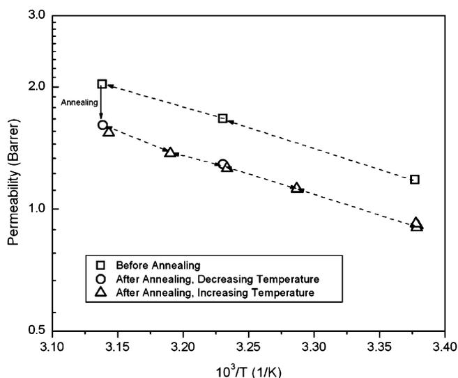
Fig. 3. The measured  $\text{CO}_2$  permeability in PLA film ( $L:D=98.3:1.7$ ) during annealing procedure.
