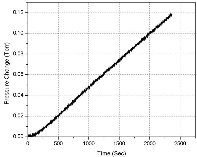
Fig. 8. Time-lag plot for O<sub>2</sub> permeation in PLA ( $L:D=80:20$ ). Temperature is 22.8 °C.
