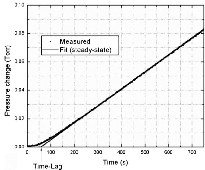
Fig. 2. Typical time lag for  $N_2$  permeation in LDPE. The measurement was conducted as a verification of the apparatus.
