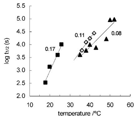
**Figure 4.** Half-times ( $t_{1/2}$ ) for the isothermal crystallization induced-gelation process as a function of the crystallization temperature, for oils A (■), B (◇), and C (▲). Lines are guides to the eyes, and the inserted numbers are the corresponding slopes.
