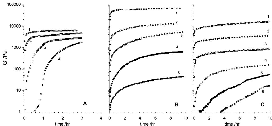
**Figure 1.** Representative cure curves showing the time dependence of the storage modulus ( $G'$ ) during isothermal crystallization for different quenching temperatures: (A) Oil A: 1, 18 °C; 2, 20 °C; 3, 24 °C; and 4, 26 °C. (B) Oil B: 1, 32 °C; 2, 36 °C; 3, 38 °C; 4, 40 °C; and 5, 42 °C. (C) Oil C: 1, 35 °C; 2, 40 °C; 3, 45 °C; 4, 48 °C; 5, 50 °C; and 6, 52 °C.
