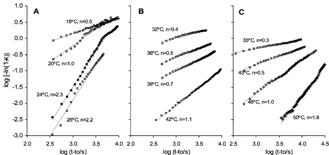
**Figure 2.** Avrami plots for oils A, B, and C, respectively (according to eqs 1 and 2). Also shown are the Avrami exponents obtained for selected curing temperatures. To illustrate the comparison among oil samples on the basis of equivalent supercooling degree, one may consider oil A at 20 °C, oil B at 32 °C, and oil C at 48 °C, which correspond to a supercooling degree of  $\Delta T \approx 25$  °C.
