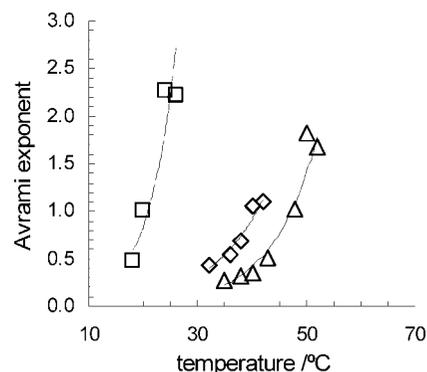
**Figure 3.** Plot of the Avrami exponent ( $n$ ) as a function of crystallization temperature, for oils A ( $\square$ ), B ( $\diamond$ ), and C ( $\triangle$ ).
