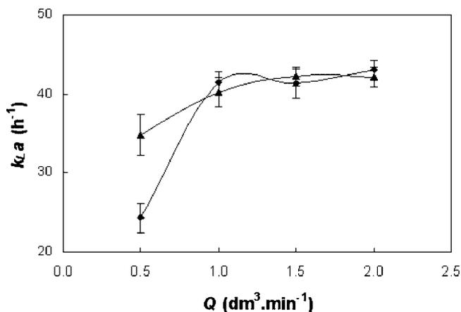
**Figure 2.** Influence of the working medium volume in the  $k_{La}$  values with pure water, at agitation rate of 250 rpm, and with impeller type A, as a function of the aeration rate. Working volume: (◆) 1.0 dm<sup>3</sup>; (▲) 1.5 dm<sup>3</sup>.
