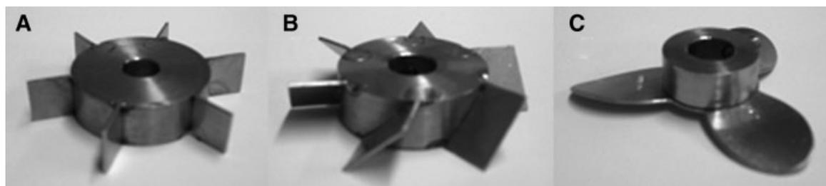
**Figure 1.** Impeller types used (A: Rushton turbine with six vertical blades; B: Pitched Blade (Axial Flow) Turbine with six blades; C: Marine type propeller with three blades).
