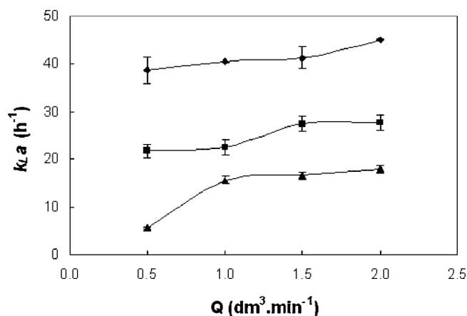
**Figure 3.** Influence of impeller position in the  $k_{La}$  values in a system with water and PFC with a volume fraction of 0.20, agitated at 250 rpm, and with impellers type B, as a function of the aeration rate: (◆) Position 1:  $h_1=3.5$  cm,  $h_2=3.0$  cm; (▲) Position 2:  $h_1=6.5$  cm,  $h_2=1.0$  cm; (■) Position 3:  $h_1=3.5$  cm,  $h_2=1.0$  cm.
