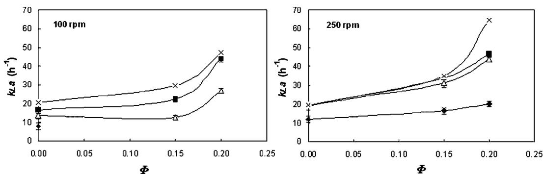
**Figure 6.** Influence of the PFC volume fraction ( $\phi$ ) in the  $k_La$  values with YPD medium, with impellers type A, with agitation rates of 100 and 250 rpm, and at different aeration rates,  $\text{dm}^3 \cdot \text{min}^{-1}$ : ( $\blacklozenge$ ) 0.5; ( $\triangle$ ) 1.0; ( $\blacksquare$ ) 1.5; ( $\times$ ) 2.0.
