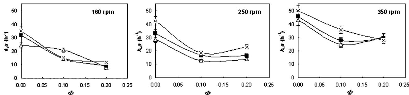
**Figure 7.** Influence of olive oil volume fraction ( $\phi$ ) in the  $k_La$  values with water, with impellers type A, with agitation rates from 160 to 350 rpm, and at different aeration rates,  $\text{dm}^3 \cdot \text{min}^{-1}$ : ( $\triangle$ ) 1.0; ( $\blacksquare$ ) 1.5; ( $\times$ ) 2.0.
