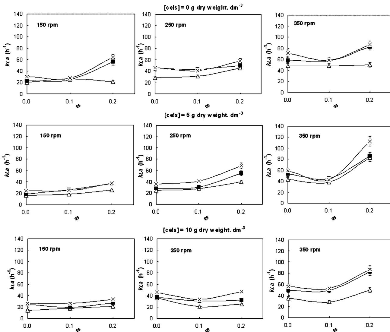
**Figure 8.** Influence of the PFC volume fraction ( $\Phi$ ) in the  $k_La$  values with YPD medium, with no cells or with two inactive cell concentrations, with impellers type A, agitation rates from 160 to 350 rpm, and at different aeration rates,  $\text{dm}^3 \cdot \text{min}^{-1}$ : ( $\Delta$ ) 1.0; ( $\blacksquare$ ) 1.5; ( $\times$ ) 2.0.
