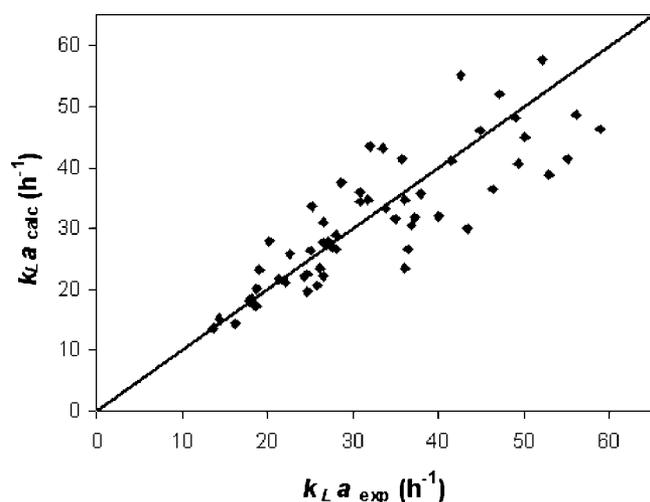
**Figure 9.** Correlation between the experimental and calculated values of  $k_L a$  for YPD medium, inactive cells, with and without PFC, agitation rates from 160 to 350 rpm and aeration rates from 1.0 to 2.0  $\text{dm}^3 \cdot \text{min}^{-1}$  ( $k_{L a \text{ exp}}$ ,  $k_{L a \text{ exp}}$  experimental values), ( $k_{L a \text{ calc}}$ ,  $k_{L a \text{ calc}}$  calculated value).
