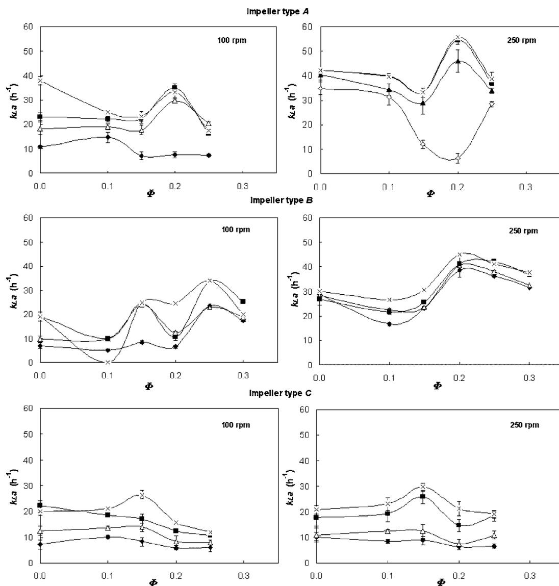
**Figure 5.** Influence of the PFC volume fraction ( $\Phi$ ) in the  $k_La$  values with water, with the three impellers type, with agitation rates of 100 and 250 rpm, and at different aeration rates,  $\text{dm}^3 \cdot \text{min}^{-1}$ : ( $\blacklozenge$ ) 0.5; ( $\blacktriangle$ ) 1.0; ( $\blacksquare$ ) 1.5; ( $\times$ ) 2.0.
