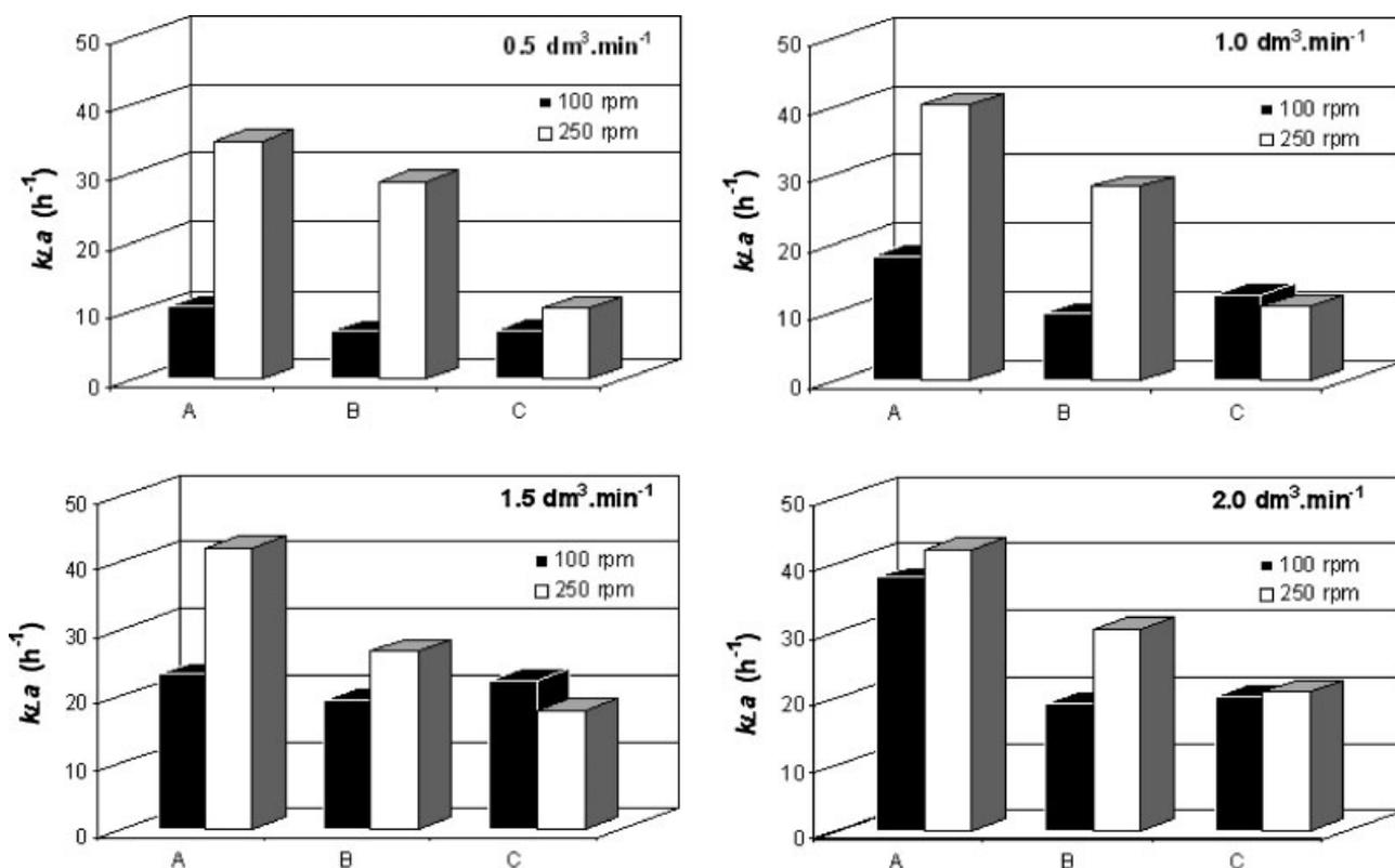
**Figure 4.** Influence of the impeller kind in the  $k_{La}$  values using pure water at 100 and 250 rpm agitation rate and at aeration rates from 0.5 to 2.0  $\text{dm}^3 \cdot \text{min}^{-1}$ . (A: Rushton turbine with six vertical blades; B: Pitched Blade (Axial Flow) Turbine with six blades; C: Marine type propeller with three blades).
