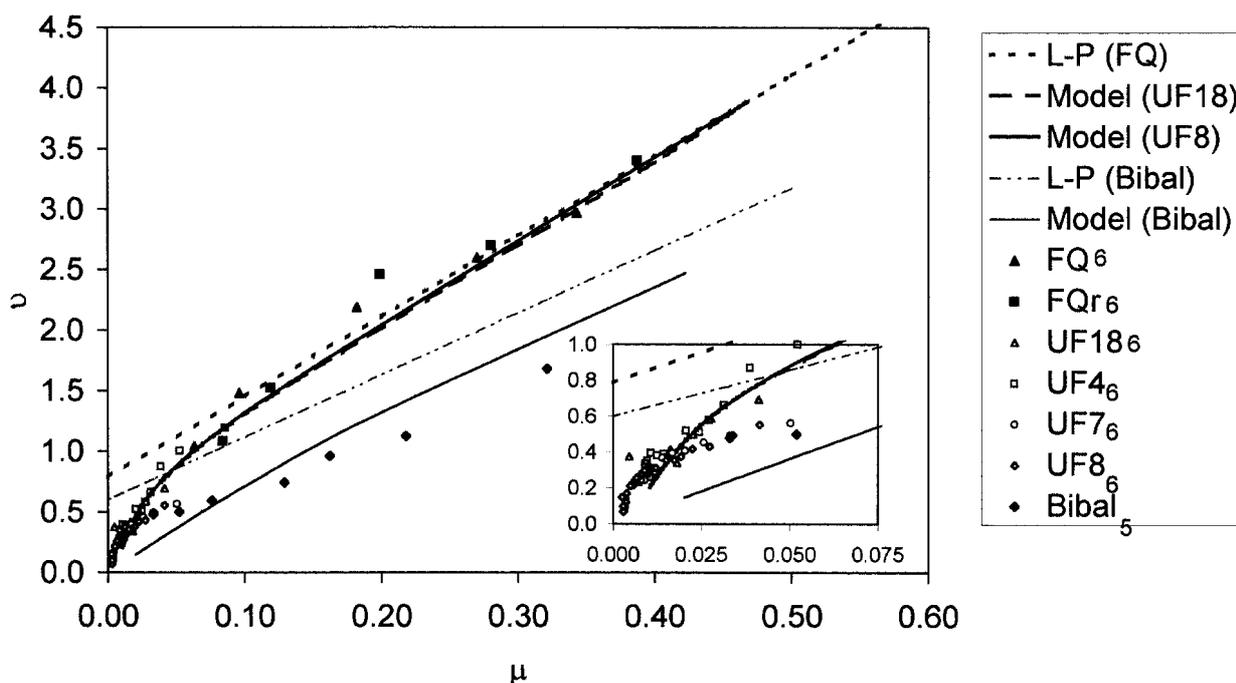
**Figure 6.** Comparison of  $v_{ap}$  and  $\mu_{ap}$  with model results and the Luedeking–Piret relationship ( $v$  vs  $\mu$ ) for the studied fermentations. FQ and FQr are the chemostat fermentations used by Xavier,<sup>6</sup> to obtain the Luedeking–Piret parameters.
