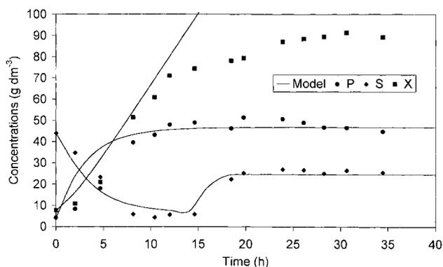
**Figure 4.** Comparison between experimental data on substrate (S), product (P) and *Lactococcus cremoris* (X) concentrations and the model results for Bibal *et al.*  $D = 1.05\text{h}^{-1}$ .
