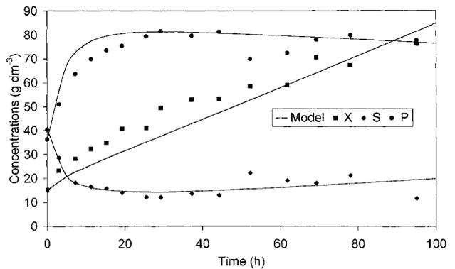
Figure 2. Comparison between experimental data of substrate ( $S$ ), product ( $P$ ) and *Lactobacillus rhamnosus* ( $X$ ) concentrations and the model results for UF7.  $D = 0.2 \text{ h}^{-1}$ .
