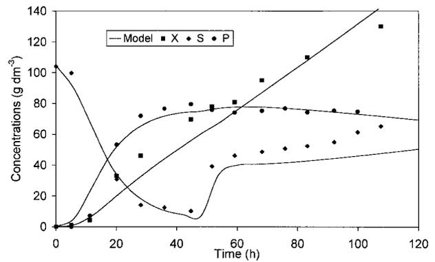
Figure 1. Comparison between experimental data of substrate ( $S$ ), product ( $P$ ) and *Lactobacillus rhamnosus* ( $X$ ) concentrations and the model results for UF18.  $D = 0.4 \text{ h}^{-1}$ .
