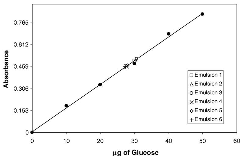
Fig. 4. Standard plot for absorbance at 540 nm as function of the glucose present (Exp. data, ●; solid line, linear regression) and samples interpolation.
