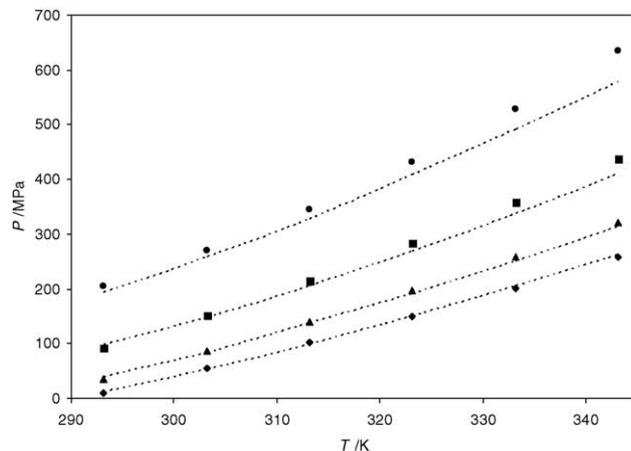
Fig. 7. Experimental data and correlation by the Eq. (14) of system {*n*-hexadecane (1) + *n*-hexane (2)} at constant mole fractions. (●) 0.1000; (■) 0.2765; (▲) 0.6002; (◆) 0.9543; dotted line correlation.
