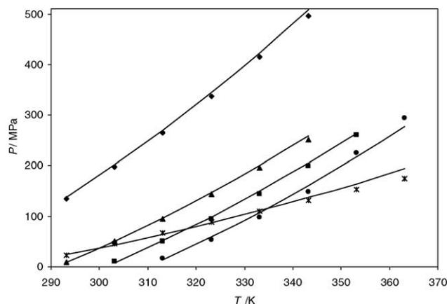
Fig. 2. Modelling of pure components data using the predictive method proposed on this work (Eq. (11)). (♦)  $n$ -tridecane, (▲)  $n$ -hexadecane, (■)  $n$ -octadecane, (●)  $n$ -eicosane, (×) cyclohexane, (—) prediction.
