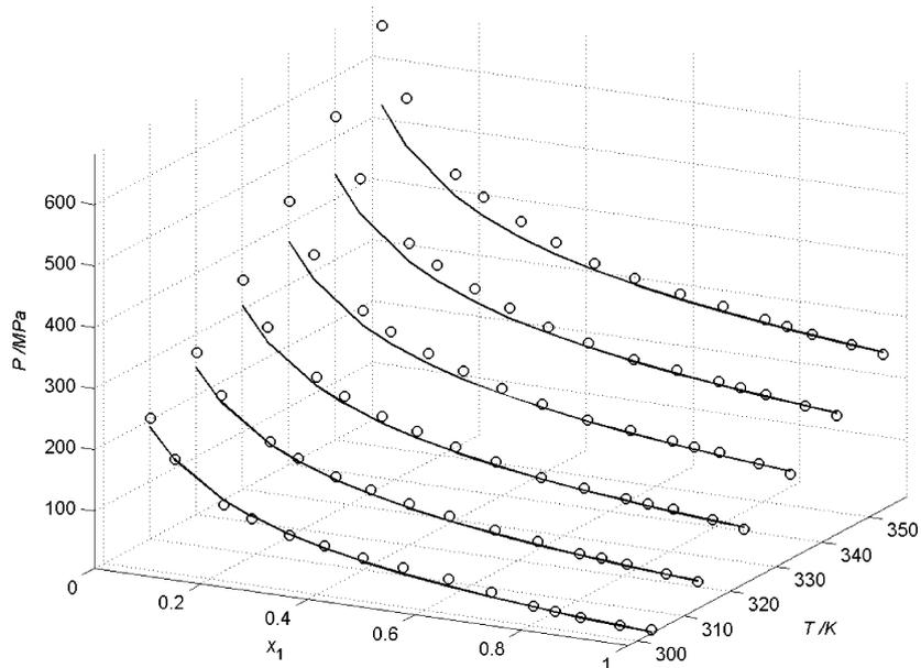
Fig. 8. Prediction and experimental data of {*n*-octadecane (1) + *n*-hexane (2)} system.
