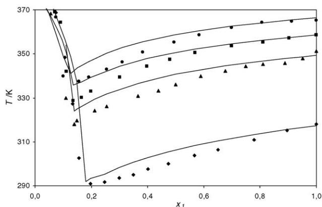
Fig. 3. Prediction of freezing temperatures (within the range of experimental temperature) of systems { $n$ -alkane (1) + cyclohexane (2)} at the pressure  $P = 300$  MPa and comparison with experimental data [20]. (◆)  $n$ -tridecane, (▲)  $n$ -hexadecane, (■)  $n$ -octadecane, (●)  $n$ -icosane, (—) prediction.
