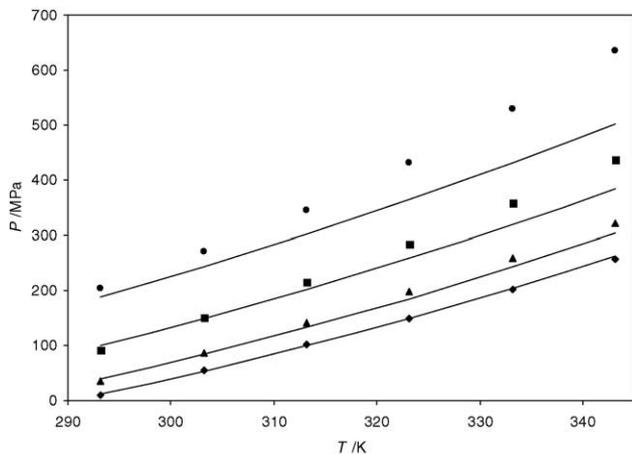
Fig. 6. Experimental data and prediction by Eq. (11) of system {*n*-hexadecane (1) + *n*-hexane (2)} at constant mole fractions. (●) 0.1000; (■) 0.2765; (▲) 0.6002; (◆) 0.9543; solid line (—) prediction.
