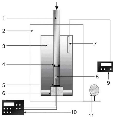
Fig. 1. Scheme of the high-pressure device: (1) piston; (2) thermstate; (3) steel vessel; (4,5) metallic rings; (6) high-pressure stopper with wires; (7) Pt(100) thermocouple; (8) manganine gauge; (9) digital thermometer; (10) digital multimeter; (11) mechanical indicator of position.
