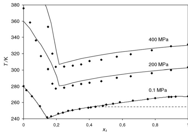
Fig. 4. Prediction of freezing temperatures of { $n$ -tridecane (1) + cyclohexane (2)} system at different pressures  $P = 200$  and 400 MPa and at atmospheric pressure. Solid line at 0.1 MPa describing experimental points are calculated by Wilson equation; dotted line exhibits solid–solid phase transition.
