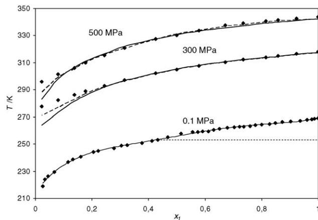
Fig. 5. Freezing temperatures of { $n$ -tridecane (1) +  $n$ -hexane (2)} system at different pressures  $P = 300$  and 500 MPa and at atmospheric pressure. Comparison of prediction Eq. (11), (solid line) and correlation with Eq. (14) (dashed line). Dotted line exhibits solid–solid phase transition.
